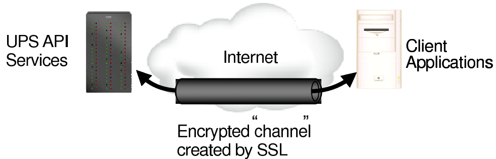
Figure 2: SSL creates a secure channel across a network and protects confidential communications using that channel.
