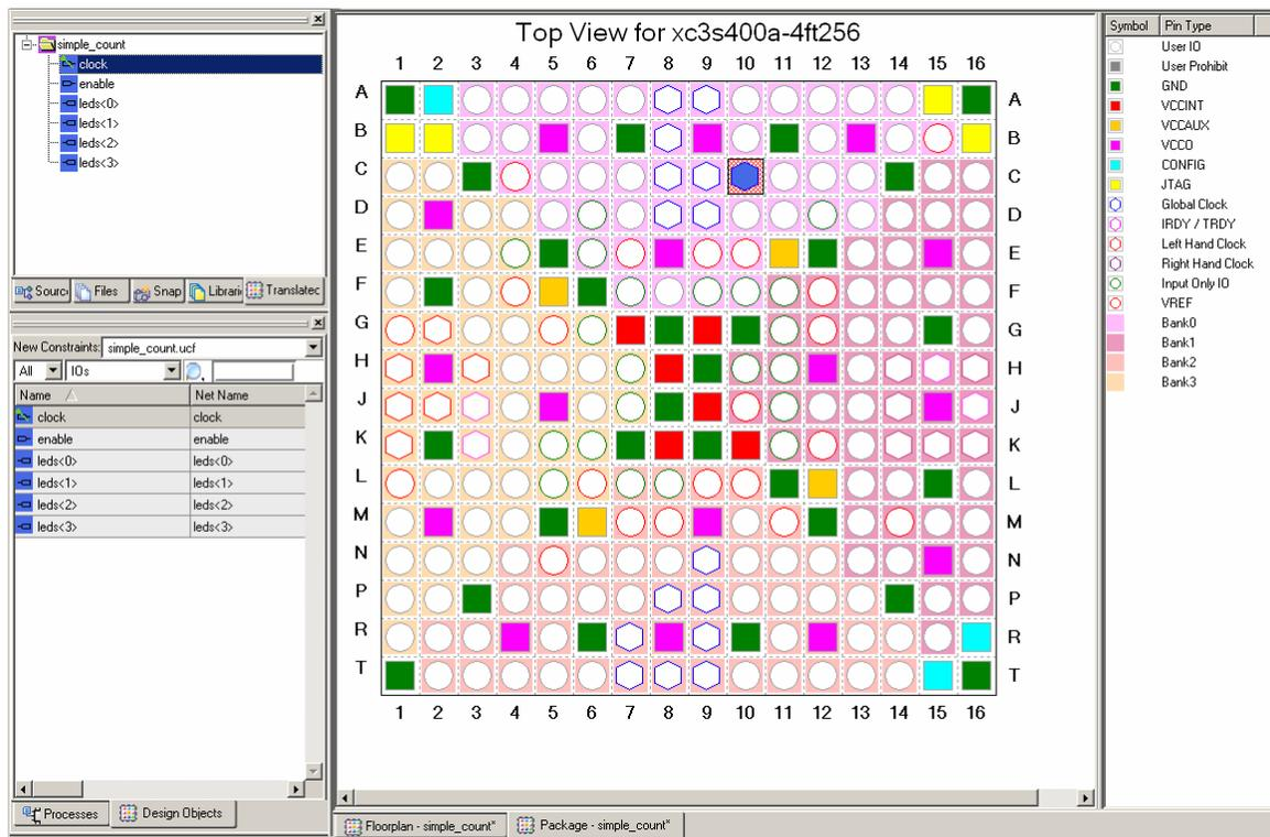
Note that your 16 MHz clock signal goes into one of the 16 Global Clock pins on the FPGA. Clock input signals should connect to global clock pins to utilize the internal global clock buffers inside the FPGA.
