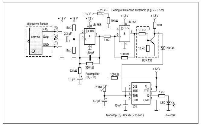
Note: The influence of fluorescent light interference (100 Hz carrier) has to be reduced by the installation of an additional 100 Hz notch filter.
