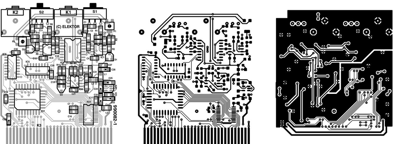
Figure 8. PCB design for the double-sided through-plated cartridge board.
