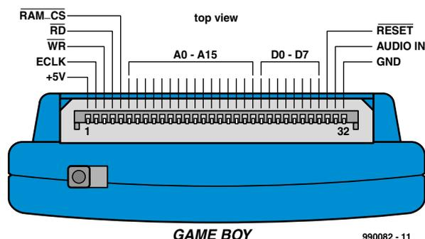
Figure 1. Gameboy card edge connector (end view of ROM cartridge).
