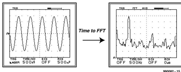
Figure 5. FFT of 1 kHz 0 dB sinewave.
