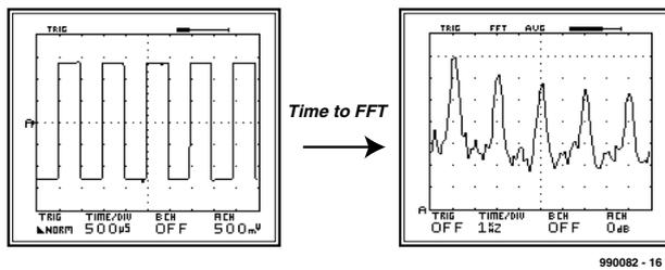
Figure 6. FFT of 1 kHz 0 dB squarewave.
