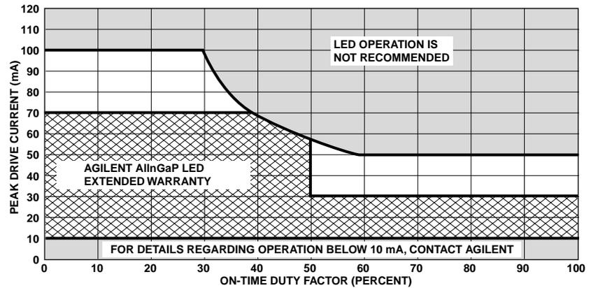
Figure 6. Agilent Technologies AllnGaP LED Extended Warranty Pulsed Current Operating Range
