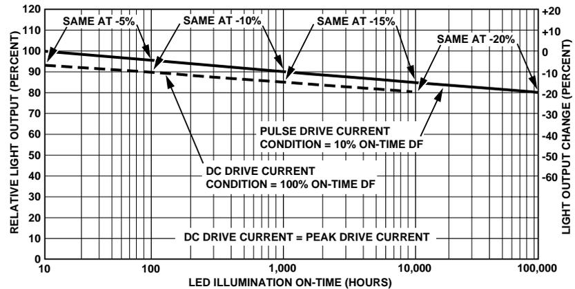
**Figure 1. Comparison of Hypothetical LED Degradation of -5% per Decade On-Time Hours for 10% DF Pulsed Drive Condition vs. dc Drive Condition (100% DF), where dc Current Value = Peak Pulse Current Value.**
