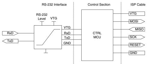
**3.1.1RS-232 Serial**<br/>InterfaceThe AVRISP uses a standard female DSUB, RS-232 port for communication with the<br/>front-end software (AVR Studio). It supports communication of 115200 baud.
