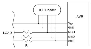
**3.4.4 RESET** To enter programming mode, AVRISP needs to pull RESET low. It is important that the external pull-up resistor on RESET pin is not so strong that it forces (holds) the pin high. To avoid this problem it is recommended that the RESET pull-up resistor should be no less than 10 k $\Omega$ .
