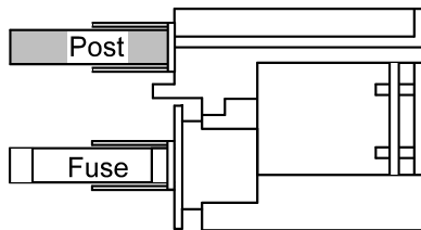
Fuse installation for 100/120 voltage
