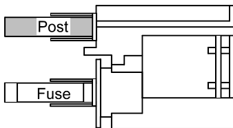
Fuse installation for 100/120 voltage
