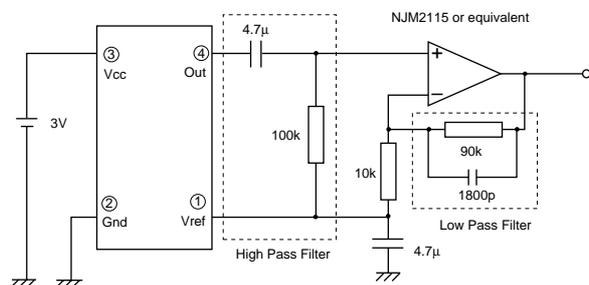
The High-pass Filter's Cut-off frequency in this circuit is approx. 0.3Hz.
