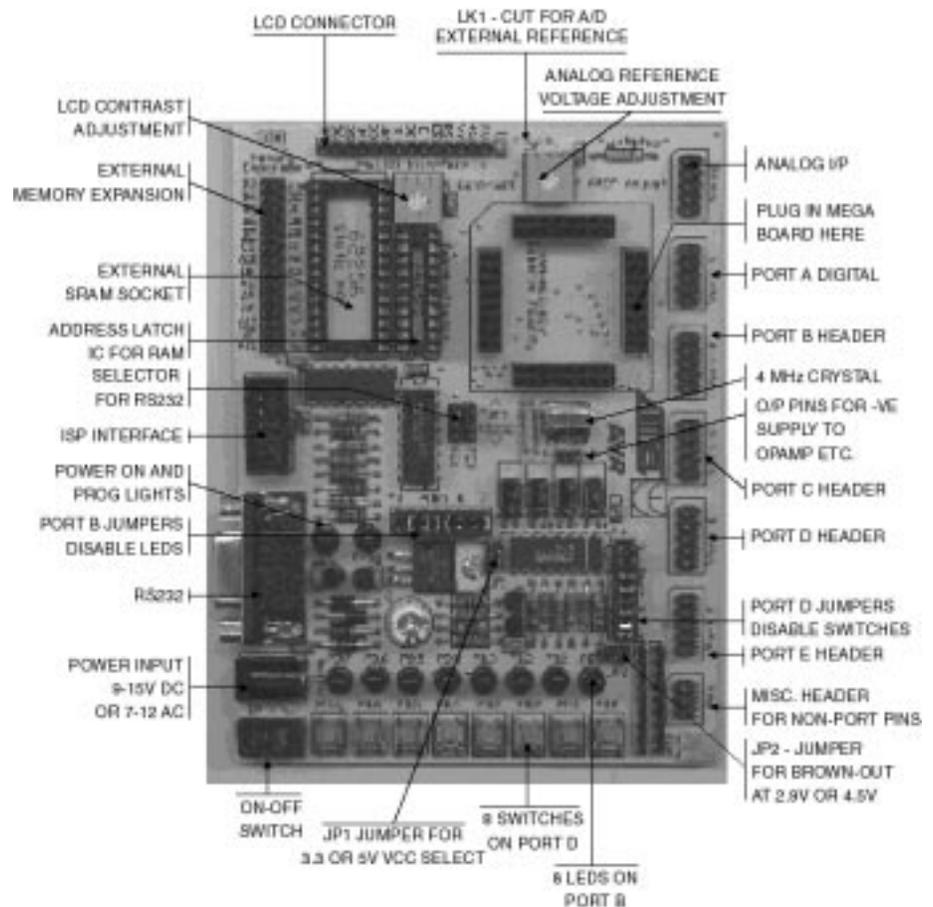
**Note:** There are a number of jumpers on the board which are used to select different operations and voltages. The default jumper settings are for programming operations at 5V JP1 Closed, with brown-out also set to 5V JP2 Open. To carry out other operations, some jumpers may have to be removed—refer to the relevant section for details. A full list of the jumpers and links are given in the table below.
