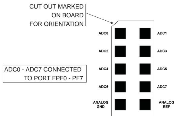
The A/D converters can use either the on-board (Internal) Voltage Reference or an external Voltage Reference.
