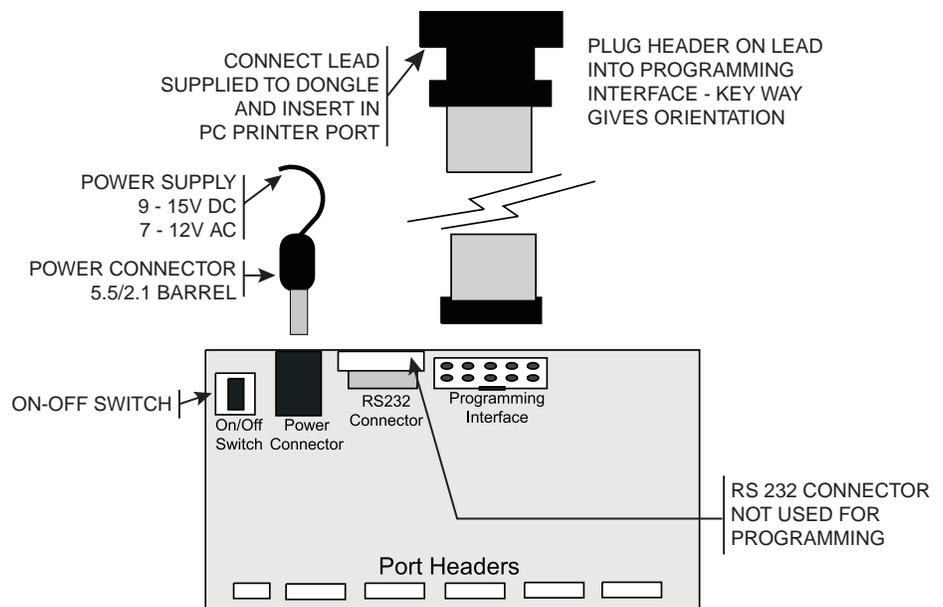
A Power Supply is required with a standard 2.1mm barrel connector. It can be AC 7 - 12V or DC 9 - 15V. The connector is inserted into the power connection socket as shown, above.
