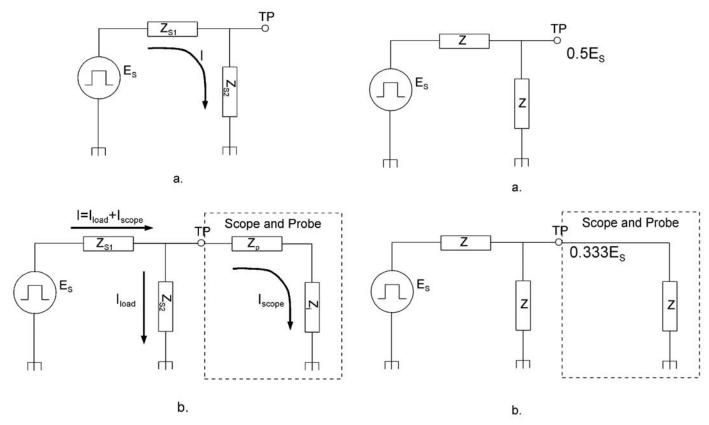
Figure 4.1. The signal being measured at the test point (TP) can be represented by a signal source and associated load impedances (a). Probing the test point adds the probe and oscilloscope impedances to the source load, resulting in some current draw by the measurement system (b).
