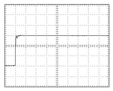
Figure 6.3. The 1 ns rise time step waveform as acquired through an ECB-to-Probe Tip Adapter.
