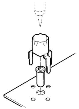
Figure 4.11. An ECB to probe-tip adaptor.
