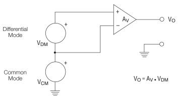
Figure 6.7. A differential amplifier has two signal lines which are differenced into a single signal that is referenced to the ground.
