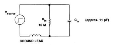
Figure 4.12. Equivalent circuit of a typical passive probe connected to a signal source.
