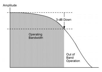
**Figure 1.5.** Probes and oscilloscopes are designed to make measurements to specification over an operating bandwidth. At frequencies beyond the 3 dB point, signal amplitudes become overly attenuated and measurement results may be unpredictable.
