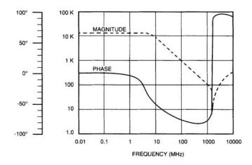
Figure 4.5. Typical input impedance versus frequency for the Tektronix P6205 Active Probe
