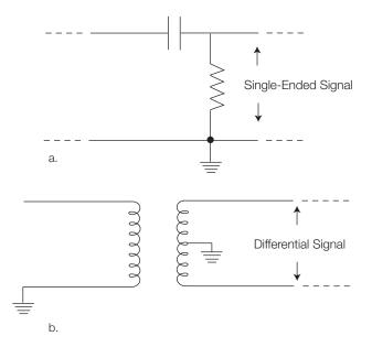
Figure 2.2. Single-ended signals are
