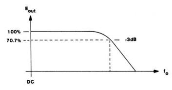
Figure 4.7. Bandwidth is defined as the frequency in the response curve where amplitude has decreased by -3 dB.
