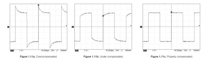
Figure 1.11a, Figure 1.11b, and Figure 1.11c. Examples of probe compensation effects on a square wave.
