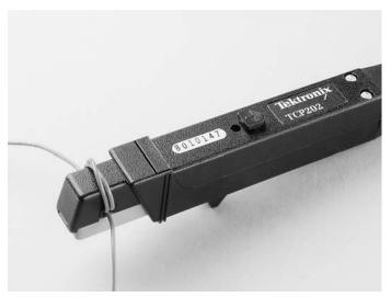
Figure 2.8. An example of a split core AC current probe. Looping n turns of the conductor through the probe increases effective snesitivity n times.
