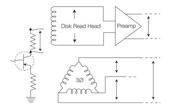
Figure 2.3. Some examples of differential signal sources.
