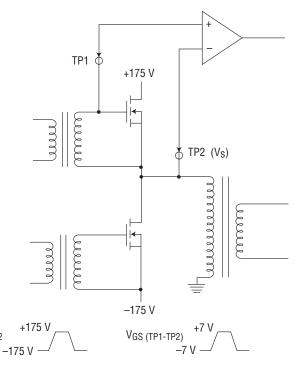
**Figure 6.8.** Differential amplifier used to measure gate to source voltage of upper transistor in an inverter bridge. Note that the source potential changes 350 volts during the measurement.
