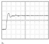
Figure 6.1a and Figure 6.1b. A fast step (1 ns Tr) has aberrations impressed on it due to use of a six-inch probe ground lead (a). These aberrations can be changed by moving the probe cable or placing a hand over the cable (b).
