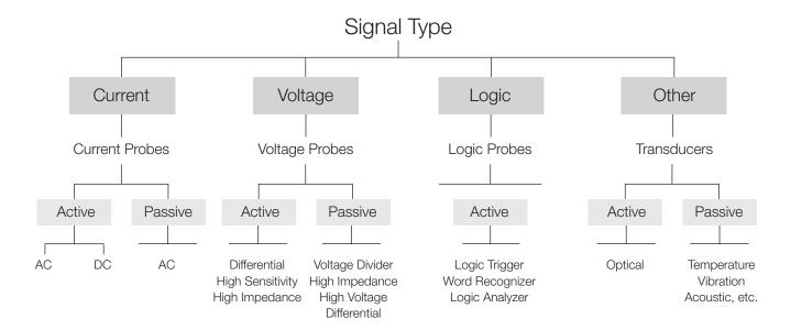
Figure 3.1. Various probe categories based on teh signal type to be measured.
