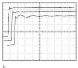
Figure 6.4a and Figure 6.4b. Examples of ground lead effects for passive probes versus active probes. The three traces on the left show the effects on the waveform of 1/2-inch, 6-inch, and 12-inch ground leads used on a passive probe. The three traces on the right show the same waveform acquired using the same ground leads, but with an active FET probe.
