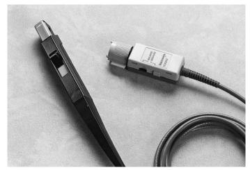
Figure 1.3c. Clamp-on Current probe.
