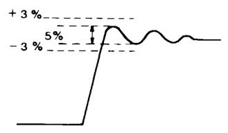
Figure 5.1. An example of measuring aberrations relative to 100% ulse height.
