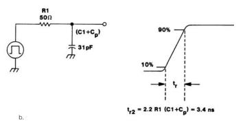
Figure 4.4a and Figure 4.4b. The added capacitance of a probe increases RC the value and increases the measured rise time.
