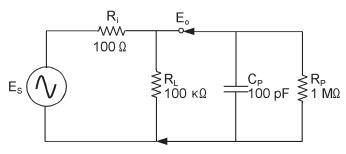
Figure 1.8. For AC signal sources, probe tip capacitance ( $C_D$ ) is the greatest loading concern. As signal frequency increases, capacitive reactance (X<sub>c</sub>) decreases, causing more signal flow through the capacitor.
