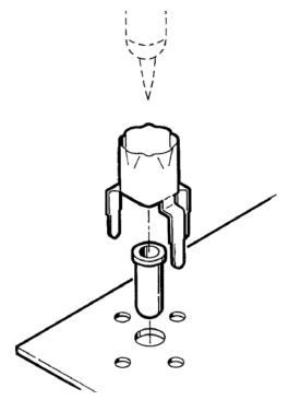
Figure 6.2. Typical ECB-to-Probe Tip Adapter installation
