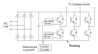
Figure 2.11. In this three-phase motor drive, all points are above the ground, making floating measurements a necessity.
