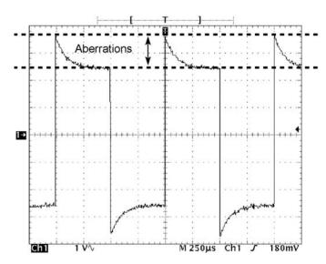
Figure 5.2. Aberrations from over compensating a probe.
