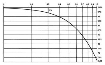
Figure 4.8. Bandwidth derating curve.
