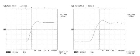
Figure 1.12a. Direct probe tip contact.
