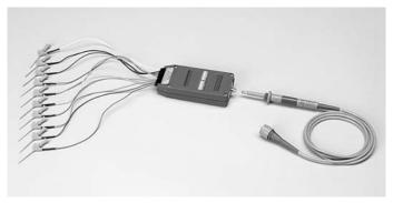
Figure 2.9. A word recognizer probe. Such probes allow oscilloscopes to be used to analyze specific data waveforms during specific logic conditions.
