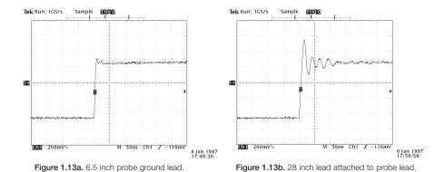
Figure 1.13a and Figure 1.13b. Extending the length of the probe ground lead can cause ringing to appear on pulses.
