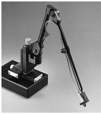
Figure 2.10. Example of a probing station designed for probing small geometry devices such as hybrid circuits and ICs.
