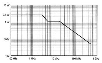
Figure 7.1. Example Derating Curve. Actual values and ranges will vary with specific products.
