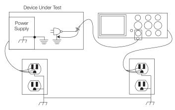
Figure 6.5. The complete ground circuit, or ground loop, for an oscilloscope, probe, and test circuit on two different power plugs.
