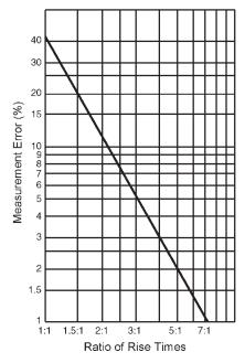
**Figure 1.6.** Rise time measurement error can be estimated from the above chart. A oscilloscope/probe combination with a rise time three times faster than the pulse being measured (3:1 ratio) can be expected to measure the pulse rise time to within 5%. A 5:1 ratio would result in only 2% error.
