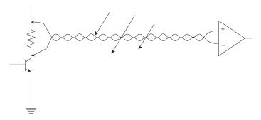
Figure 6.11. With the input leads twisted together, the loop area is very small, hence less field passes through it. Any induced voltage tends to be inthe VCM path which is rejected by the differential amplifier.
