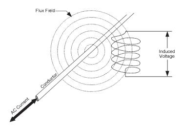
Figure 2.6. A voltage is induced across any coil that is placed in the changing flux field around a conductor which is carrying alternating current (AC).
