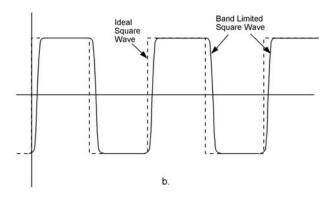
Figure 3.2. When major frequency components of a signal are beyond the measurement system bandwidth (a), they experience a higher degree of attenuation. The result is loss of waveform detail through rounding of corners and lengthening
