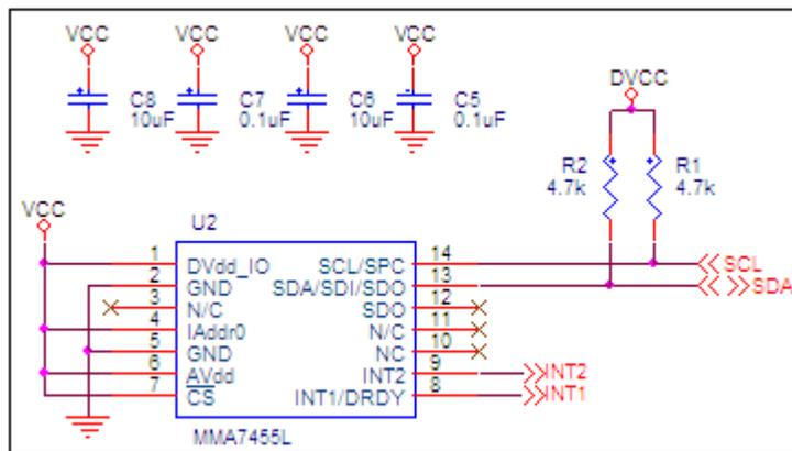
Figure 2. I<sup>2</sup>C Communication Sensor Connections
