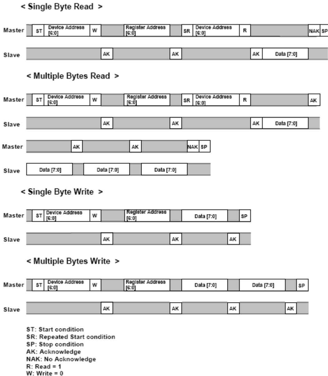
**Figure 3. IIC Read and Write Protocol Format**
