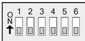
Figure 2.6. RS-485 (2-wire) Half-Duplex DIP Switch Settings
