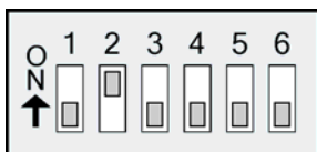
Figure 2.10. RS-485 (4-wire) and RS-422 DIP Switch Settings
