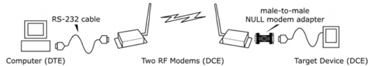
Figure B-04. Example of a Digi Radio Modem (DCE Device) connecting to another DCE device)
