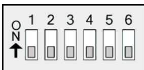
Figure 2.6. RS-485 (2-wire) Half-Duplex DIP Switch Settings
