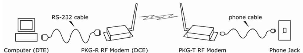
Figure 3-02. Hardware Setup - Wireless Link Method
