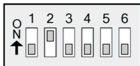
Figure 2.10. RS-485 (4-wire) and RS-422 DIP Switch Settings
