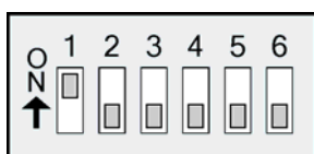
Figure 2.1. RS-232 DIP Switch Settings
