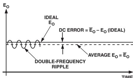
Figure 3. Output Waveform for Sine Wave Input Voltage
