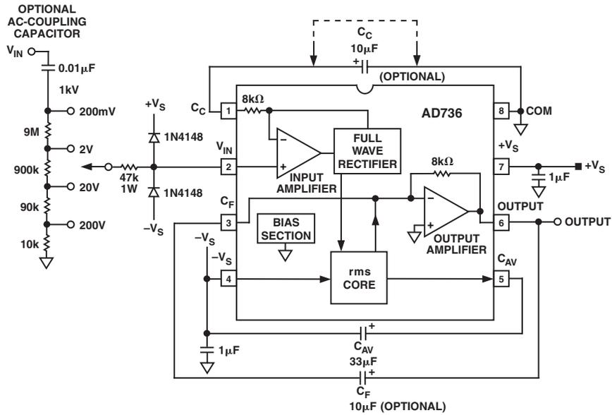
Figure 4. AD736 with a High Impedance Input Attenuator
