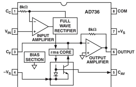
that allows the measurement of 300 mV input level while operating from the minimum power supply voltage of +2.8 V, -3.2 V. The two inputs may be used either singly or differentially.
