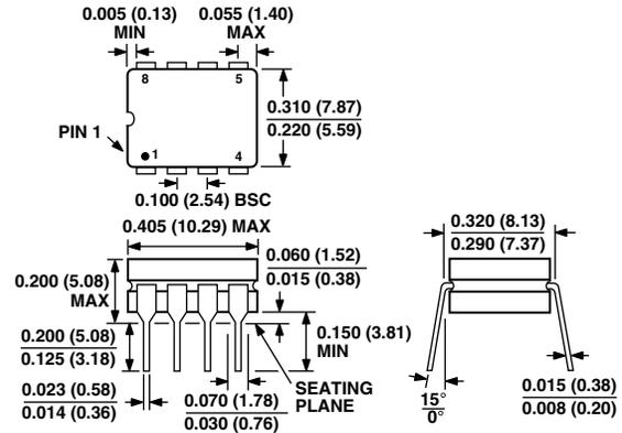
CONTROLLING DIMENSIONS ARE IN INCHES; MILLIMETERS DIMENSIONS (IN PARENTHESES) ARE ROUNDED-OFF INCH EQUIVALENTS FOR REFERENCE ONLY AND ARE NOT APPROPRIATE FOR USE IN DESIGN
