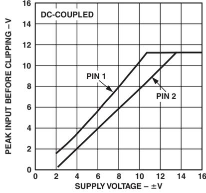
TPC 2. Maximum Input Level vs. Supply Voltage
