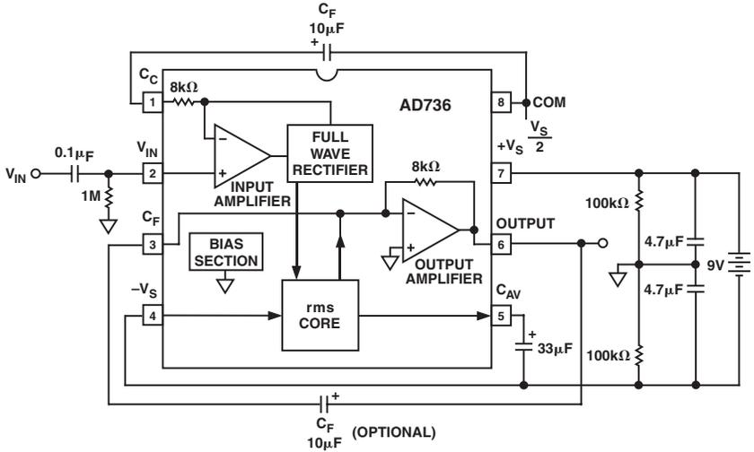
Figure 7. Battery-Powered Option
