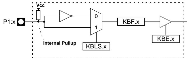
**Figure 28.** Keyboard Input Circuitry
