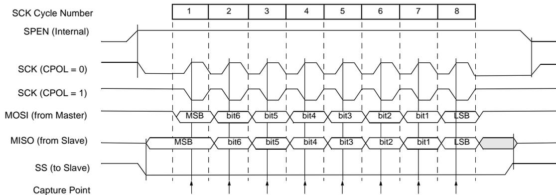
**Figure 33. Data Transmission Format (CPHA = 1)**
