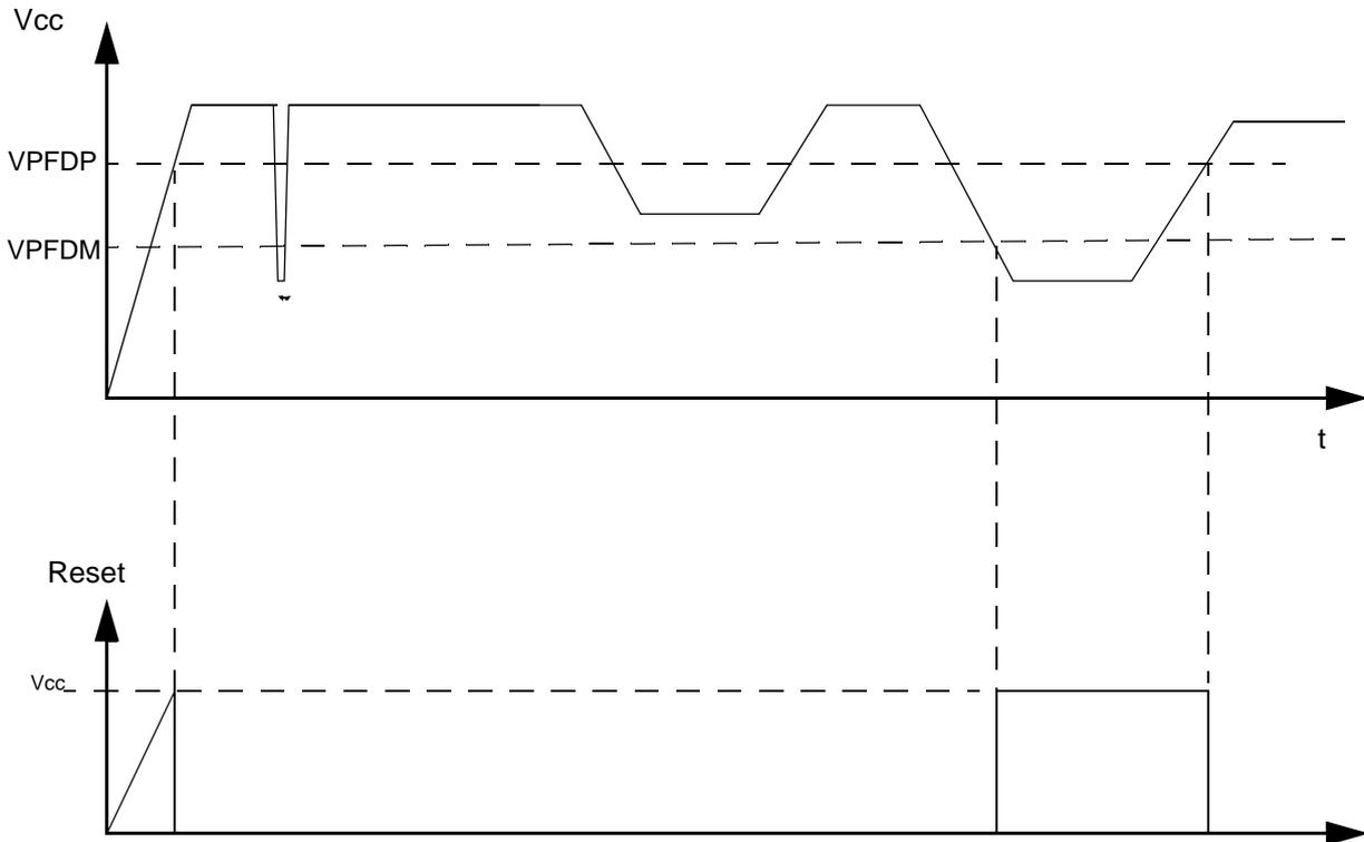
When the power is applied, the Power Monitor immediately asserts a reset. Once the internal supply after the voltage regulator reach a safety level, the power monitor then looks at the XTAL clock input. The internal reset will remain asserted until the Xtal1 levels are above and below  $V_{IH}$  and  $V_{IL}$ . Further more. An internal counter will count 1024 clock periods before the reset is de-asserted.
