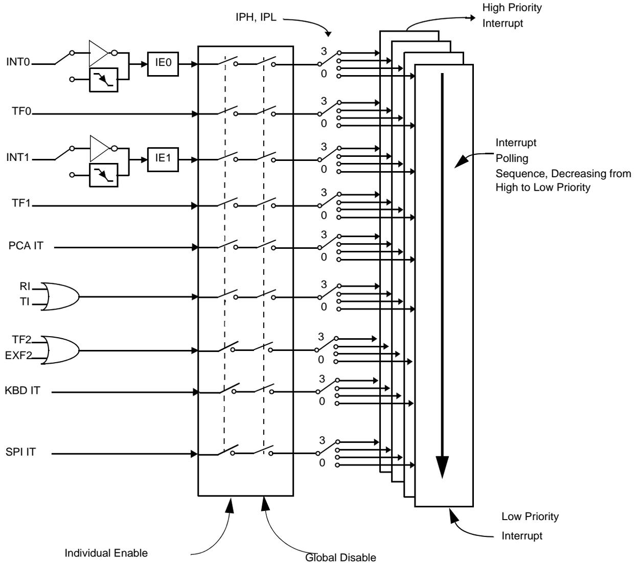
Each of the interrupt sources can be individually enabled or disabled by setting or clearing a bit in the Interrupt Enable register (Table 54 and Table 56). This register also contains a global disable bit, which must be cleared to disable all interrupts at once.
