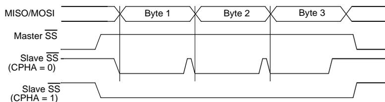
As shown in Figure 32, the first SCK edge is the MSB capture strobe. Therefore, the Slave must begin driving its data before the first SCK edge, and a falling edge on the SS pin is used to start the transmission. The SS pin must be toggled high and then low between each Byte transmitted (Figure 34).
