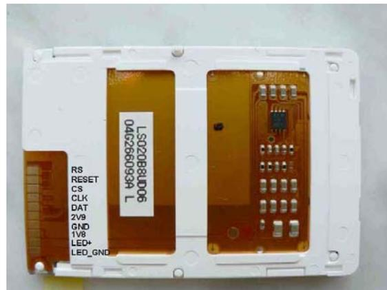
The display interface was measured using a HP (Agilent) 16-channel digital oscilloscope. (unfortunately a logic analyser was not available)
