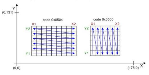
For partial writing to the memory the commands below are used. The start corner (X1,Y1) and the end corner (X2,Y2) have to be defined. X2 has to be larger or equal X1, Y2 has to be larger or equal Y1.
