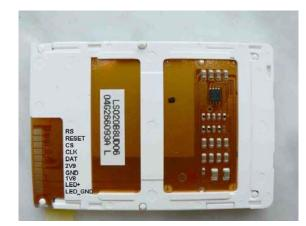
The display interface was measured using a HP (Agilent) 16-channel digital oscilloscope. (unfortunately a logic analyser was not available) The display commands and data are written in a 16-bit format like the example on the picture. A data bit is latched with the rising edge of the clock signal by the display controller.
