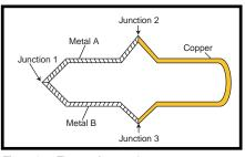
Figure 1c—The act of connecting a measurement system made of copper introduces two parasitic thermocouples.
