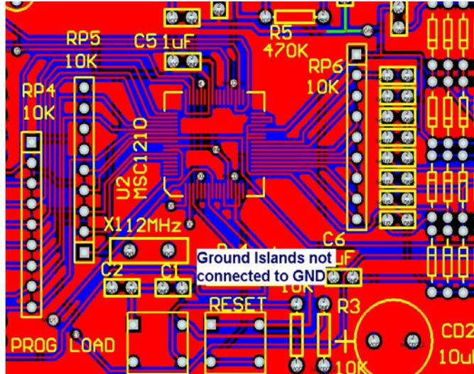
These top planes seem to be just an area fill for the gaps in the traces. When the plane areas on the top layer are not connected to the ground plane on the bottom, that means that the ground plane on the bottom doesn't have a continuous path available for current. If these top ground planes were connected to the bottom ground plane, the ground return currents would have a lower inductance path.
