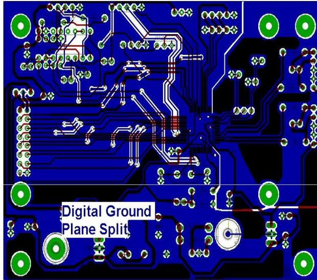
Analog and Digital sections separated with ground planes on both the bottom and the top. But the bottom ground plane is seriously split so that the ground return currents can't flow close to the source signal wires.
