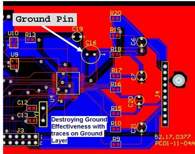
Here we see serious splits in the bottom ground plane. A close examination will also show that the traces that are splitting the ground plane are actually also ground signals.
