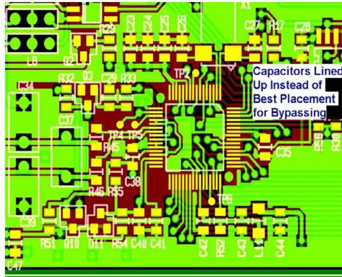
If we position capacitors and components with an order and goal of symmetry, the results could be unnecessary inductance and resistance that are introduced which will reduce the performance of the system.
