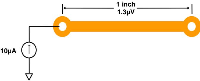
The diagram illustrates a PCB layout tip for high-resolution measurements. It shows a 10µA current source connected to a 1-inch trace. The voltage drop across the trace is 1.3µV. The trace is highlighted in orange.
