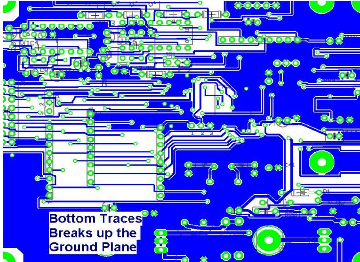
This shows the problem of using a digital PCB layout for an analog board. It simplifies the routing for most of the traces on each layer to go one direction, but that might lead to inefficiencies in the ground return currents and an unnecessary increase in inductance. Remember, inductance is defined by the size of the loop for the current.
