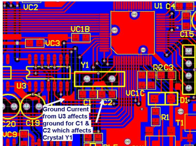
The ground current from U3 was routed to the ground point for the crystal (Y1) capacitors and then to the rest of the ground in the system. This caused a significant effect on the oscillator and made the clock very unstable.
