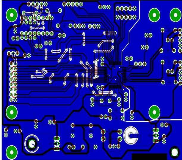
A few simple changes in the routing were able to provide a much better ground return path. Larger continuous areas of ground plane translate into short return current paths and lower inductance.
