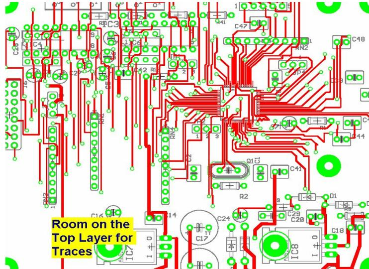
As this layer is compared with the next slide, it is evident that some of the traces could have been put on this layer so that the ground layer could have been more solid.
