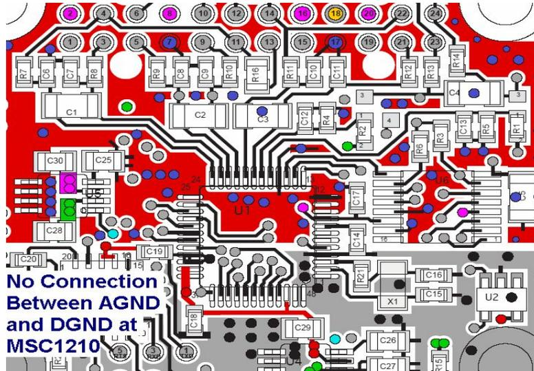
There is a good separation between the analog and digital sections, but the AGND and DGND should be connected together at the ADC.
