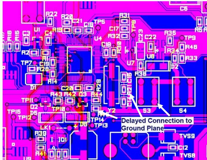
Here this board is designed with a reasonably solid ground plane and rather than connecting directly with feedthroughs to ground plane, there are large traces to a centralized ground connection point. The extra inductance and resistance, even with wide traces, will reduce the performance of the board compared to feedthroughs (or multiple feedthroughs) placed close to the component's ground connection.
