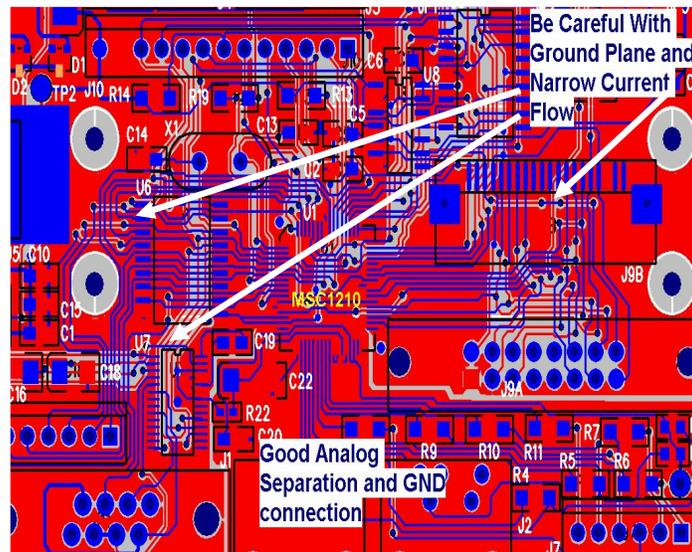
The Analog and Digital sections are nicely separated. The AGND and DGND are connected with a wide connection right at the MSC1210. But the ground plane sometimes has narrow channels for current which will increase inductance and noise. The return currents for the digital signals will want to travel under the horizontal traces, but the channels in the ground plane are generally vertical.
