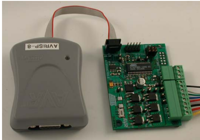
Figure 4-1 . Programming from AVR ISP programmer
