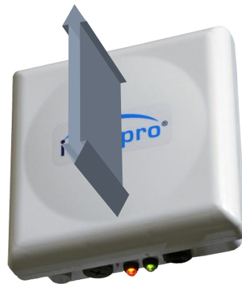
Illustration 6: Orientation of the plane of polarization of the linear antenna
