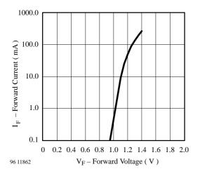
Figure 3. Forward Current vs. Forward Voltage
