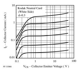
Figure 6. Collector Current vs. Collector Emitter Voltage
