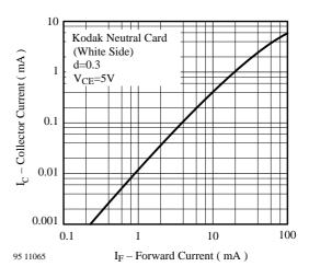
Figure 5. Collector Current vs. Forward Current
