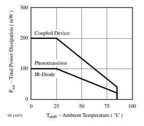
Figure 2. Total Power Dissipation vs. Ambient Temperature
