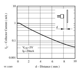
Figure 9. Collector Current vs. Distance
