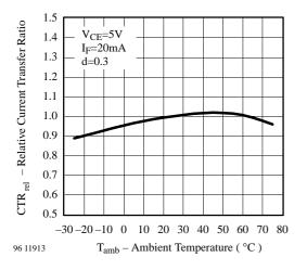
Figure 4. Rel. Current Transfer Ratio vs. Ambient Temperature
