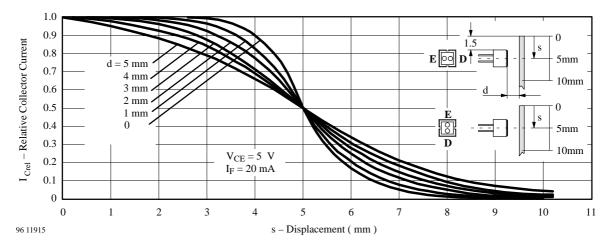
Figure 11. Rel. Collector Current vs. Displacement
