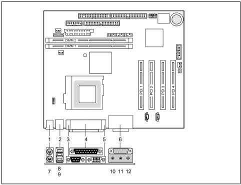
1 = PS/2 mouse port7 = PS/2 keyboard port2 = LAN port8 = USB port B3 = Serial port 19 = USB port A4 = Parallel port10 = Audio line-out5 = VGA connector11 = Audio line-in6 = Game/Midi port12 = Audio micro-in
