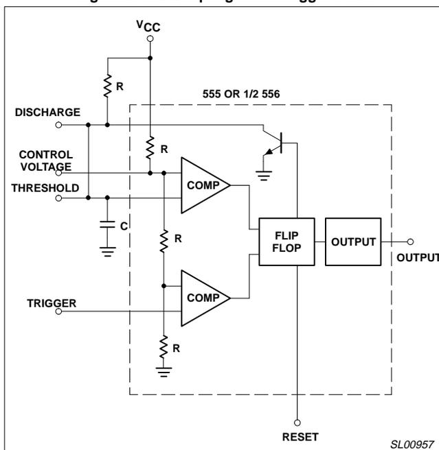
Figure 4. Monostable Operation
