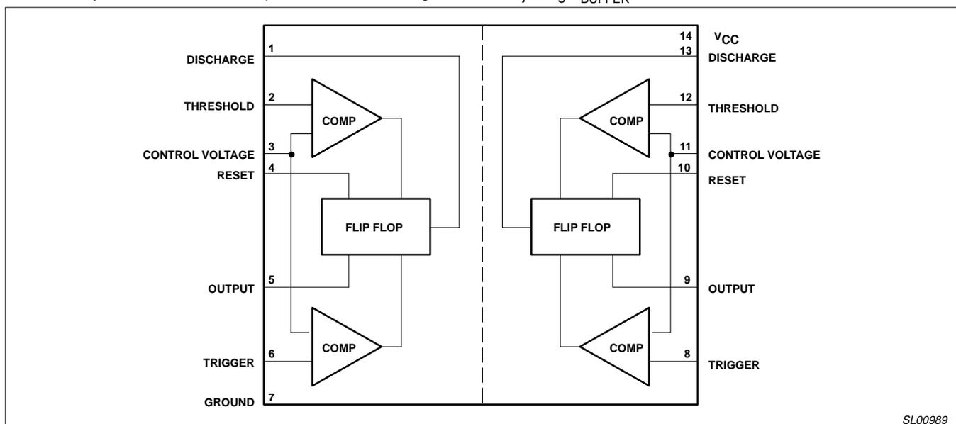
Figure 36. Block Diagram
