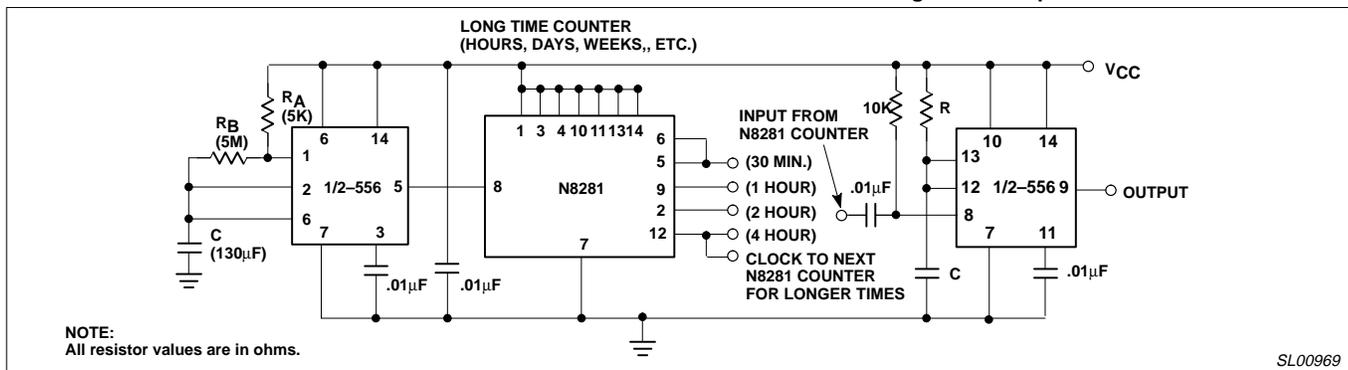
Figure 16. Method of Achieving Long Time Delays
