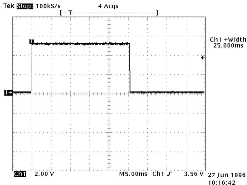
Figure 10. Jupiter GPS Receiver Time Mark Pulse Waveform
