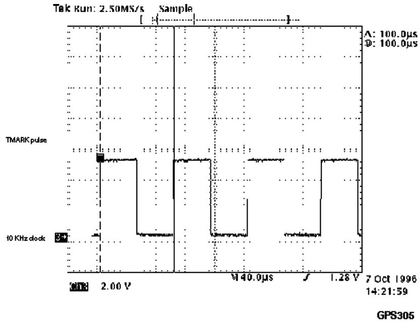
Figure 11. 10 KHz Clock/UTC TMARK Pulse Relationship
