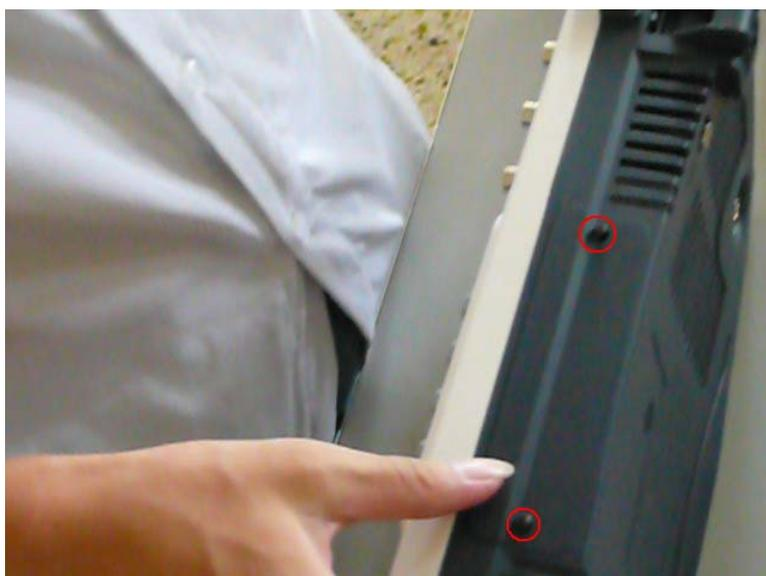
**Figure 14: Loosen the screws of battery box**
