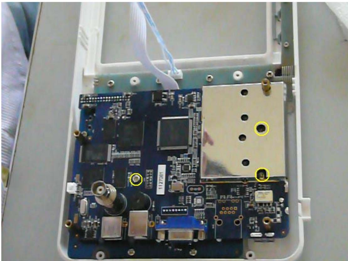
**Figure 32: Screws secure the main board**
