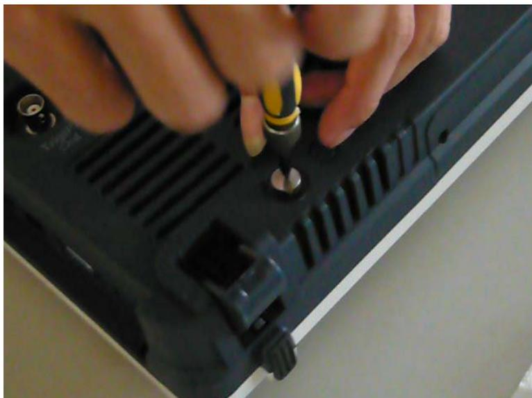
**Figure 13: Remove the Ground Connection**
