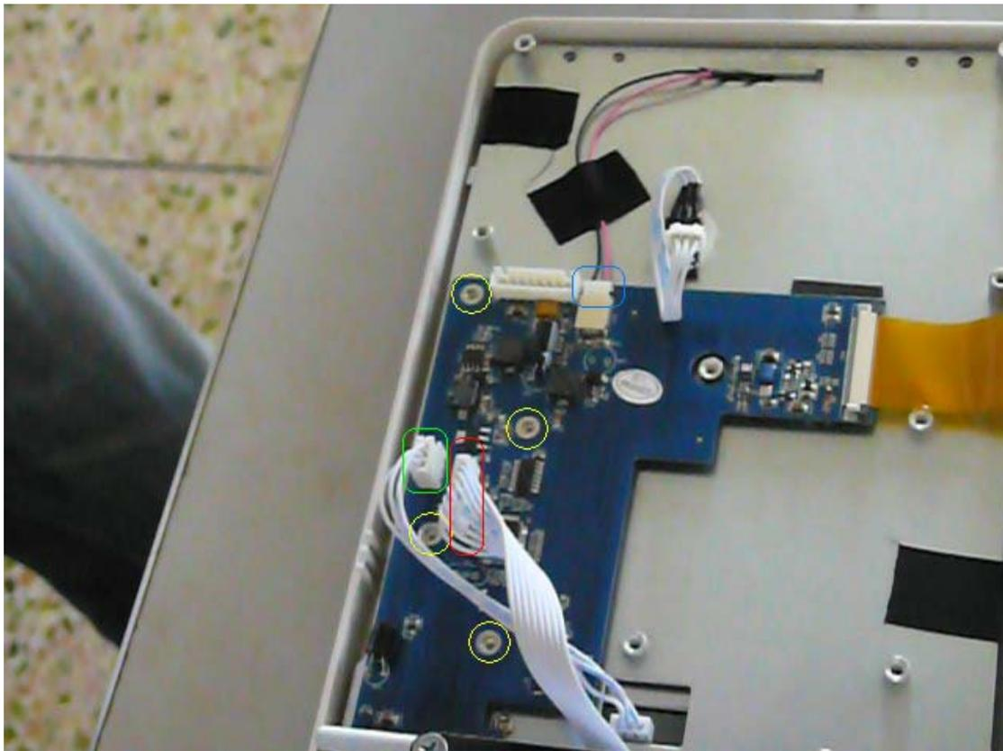
**Figure 25: Screws and cables of the adapter plate**
