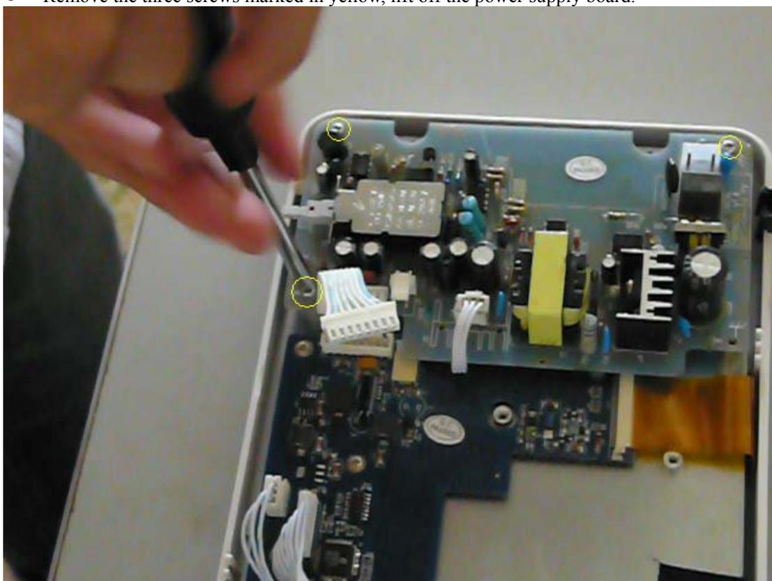
**Figure 23: Screws of power supply board**
