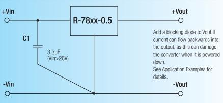
Input capacitor needed only if Vin>26VDC.
