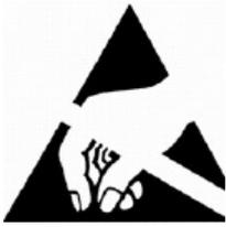
ATTENTION: LED IS AN ELECTROSTATIC SENSITIVE DEVICE. HANDLE WITH PRECAUTION.
