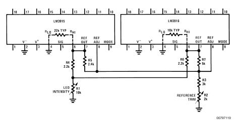
$5 \text{ mA} \leq I_{LED} \leq 28 \text{ mA}$   $V_{REF} = 5 V$
