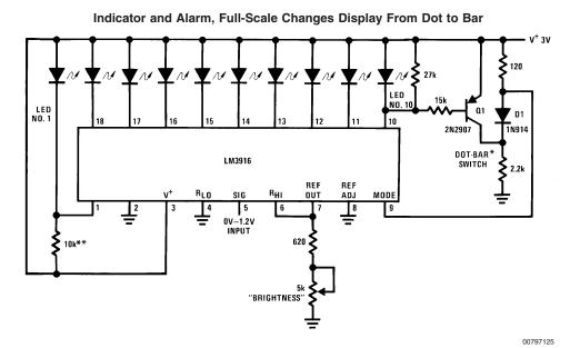
\*The input to the Dot-Bar switch may be taken from cathodes of other LEDs. Display will change to bar as soon as the LED so selected begins to light. \*\*Optional. Shunts 100 µA auxiliary sink current away from LED #1.
