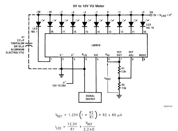
Notes: Capacitor C1 is required if leads to the LED supply are 6" or longer.
