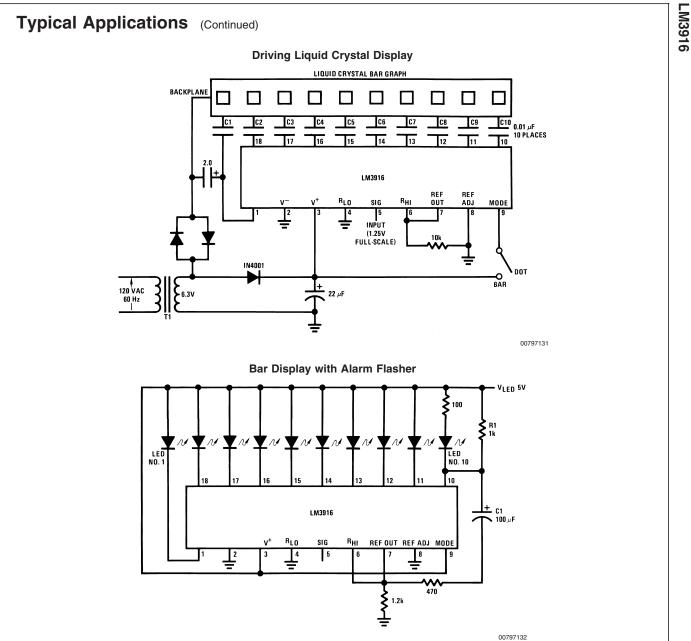
Full-scale causes the full bar display to flash. If the junction of R1 and C1 is connected to a different LED cathode, the display will flash when that LED lights, and at any higher input signal.
