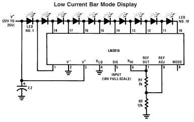
Supply current drain is only 20 mA with ten LEDs illuminated @ 16 mA.
