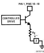
Outputs may be run in saturation with no adverse effects, making it possible to directly drive logic. The effective saturation resistance of the output transistors, equal to  $R_E$  plus the transistors' collector resistance, is about  $50\Omega$ . It's also possible to drive LEDs from rectified AC with no filtering. To avoid oscillations, the LED supply should be bypassed with a 2.2  $\mu$ F tantalum or 10  $\mu$ F aluminum electrolytic capacitor.
