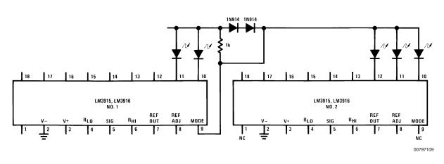
FIGURE 2. Cascading Drivers in Dot Mode with Pin 1 of Driver #2 Unused
