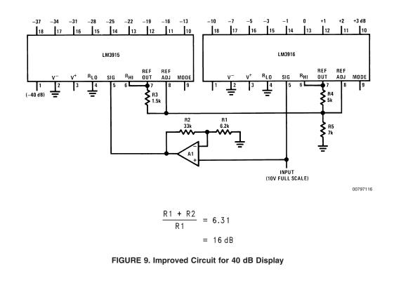
To extend this approach to get a 70 dB display, another 30 dB of amplification must be placed in the signal path ahead of the lowest LM3915. Extreme care is required as the lowest LM3915 displays input signals down to 2 mV! Several offset nulls may be required. High currents should not share the same path as the low level signal. Also power line wiring should be kept away from signal lines.
