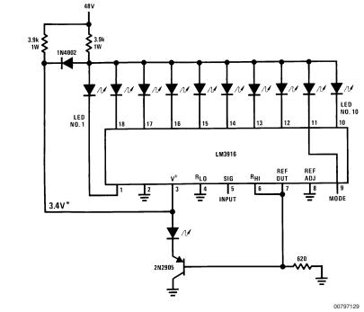
The LED currents are approximately 10 mA, and LM3916 outputs operate in saturation for minimum dissipation. \*This point is partially regulated and decreases in voltage with temperature. Voltage requirements of the LM3916 also decrease with temperature.
