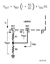
Since the 120  $\mu$ A current (max) from the adjust terminal represents an error term, the reference was designed to minimize changes of this current with V<sup>+</sup> and load changes. For correct operation, reference load current should be between 80  $\mu$ A and 5 mA. Load capacitance should be less than 0.05  $\mu$ F.
