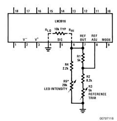
$5 \text{ mA} \leq I_{\text{LED}} \leq 28 \text{ mA} @ V_{\text{REF}} = 5V$
