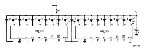
FIGURE 1. Cascading LM3914/15/16 Series in Dot Mode
