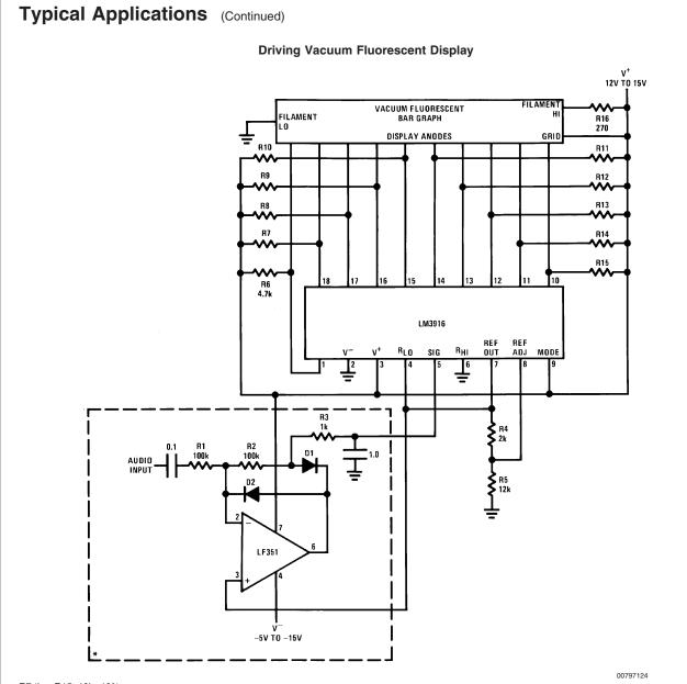
R7 thru R15: 10k±10% D1, D2: 1N914 or 1N4148 \*Half-wave peak detector. See Application Hints.
