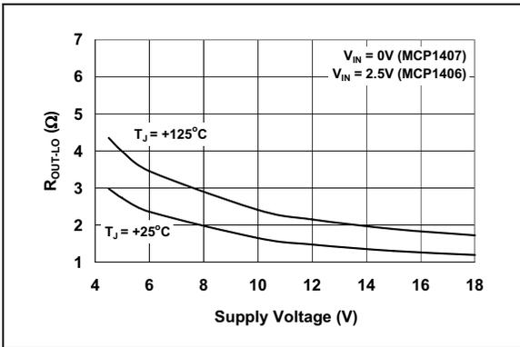
**FIGURE 2-20:** Output Resistance (Output Low) vs. Supply Voltage.
