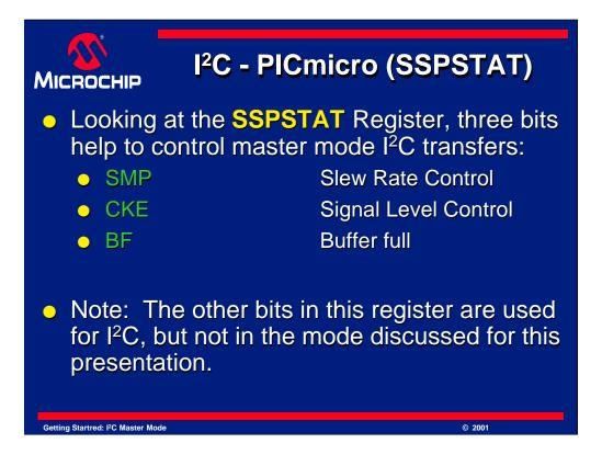
The next register that controls I<sup>2</sup>C is the SSPSTAT register. SSPSTAT stands for "Synchronous Serial Port STATus" and provides a few bits for controlling the I<sup>2</sup>C communication.
