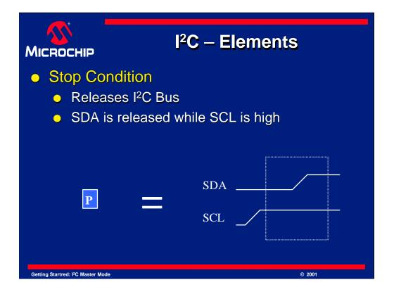
The next element we will discuss is the *Stop* condition. A start condition indicates that a device has finished its transfer on the  $I^2C$  bus and would like to release the bus. Once released other devices may use the bus to transmit data.
