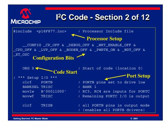
The next section is the processor setup, and indicates the processor used for the code. This example uses a PIC16F877, but many other devices could be used.
