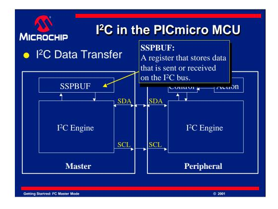
Once a byte of data has been sent to the master via I2C, it is sent to the SSPBUF register. Data to be sent on the I<sup>2</sup>C bus is also sent to the SSPBUF register, which is then sent via I<sup>2</sup>C. SSPBUF holds data to transmit or received data, depending on the current mode of the MSSP module.
