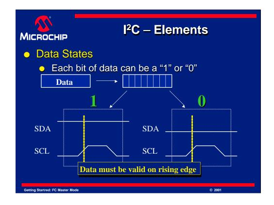
Here is a close-up view of a data block. As you can see, it contains 8 bits of data and the data is valid on the rising edge of SCL. The data then remains valid while SCL is high.
