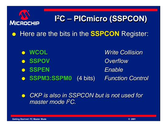
The SSPCON register is one of the 4 registers that controls the I<sup>2</sup>C engine.
