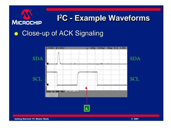
Here is a close up of the ACK pulse and the nearby spike we have mentioned. Notice that it only happens when SCL is low. Remember that data only has to be valid when SCL is high. This is part of the definition of I<sup>2</sup>C protocol. As you can see, this does happen and so the ACK will be correctly recognized. If you have trouble with your I<sup>2</sup>C system, be sure to check this. *The data must be valid when SCL goes high*.
