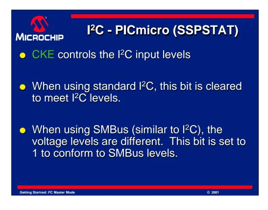
CKE controls the voltage range used by the PIC micro microcontroller when receiving  $I^2C$  signals.
