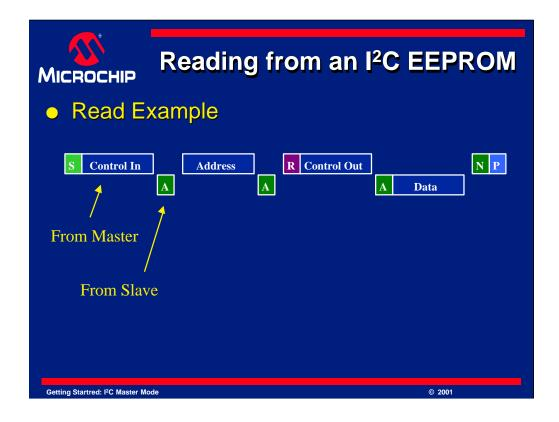
Here is an example transfer of *reading* from a small EEPROM.
