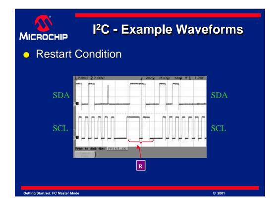
Here is a look at the restart condition. This is the first restart that occurs in the waveform. It happened after the write to the EEPROM completed and we begin the first part of the ACK polling. You can see the start and stop conditions contained within it.
