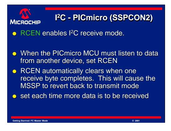
RCEN places the MSSP module into I<sup>2</sup>C receive mode.
