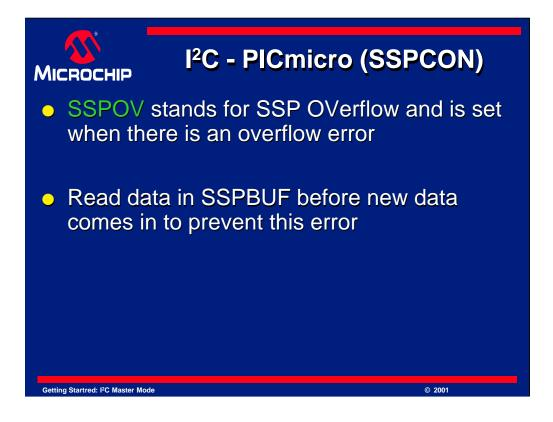
As mentioned previously, SSPOV means "Synchronous Serial Port OVerflow" and is set by the microcontroller whenever there is an overflow error.
