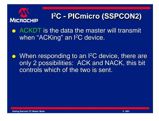
ACKDT indicates the data that will be transmitted if it is desired to send an acknowledge bit to the peripheral device. Remember, when the master reads data from a device, it must acknowledge the transfer by sending an ACK or NACK condition. This bit holds the value of the condition to be sent. If loaded with a 0, an ACK is sent, and if loaded with a 1, a NACK will be sent.
