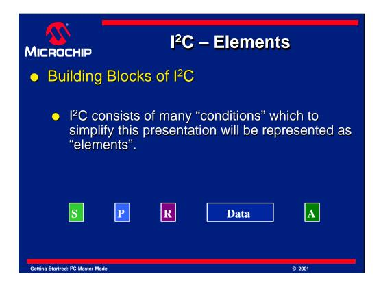
The I<sup>2</sup>C bus has a number of "conditions". These conditions indicate when a transfer is starting, stopping, being acknowledged, and other events. To simplify the explanation of I<sup>2</sup>C communications, this presentation will represent these as "elements", small colored blocks with a letter and color to represent each condition.
