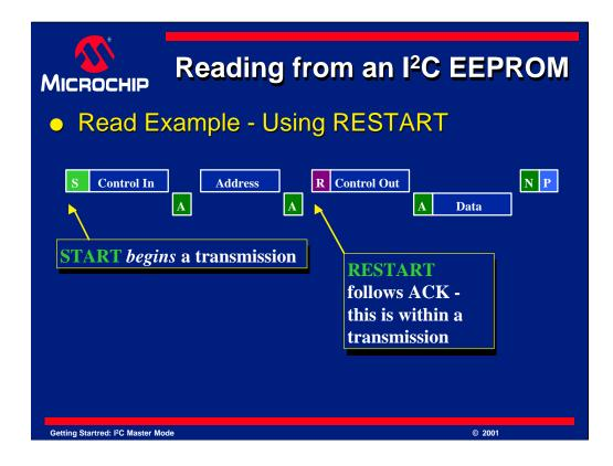
Here is another look at our EEPROM read example. As you can see, a start condition is used to begin the transfer, a restart is used in the middle of the transfer to reset the EEPROM device, and a stop ends the transfer.
