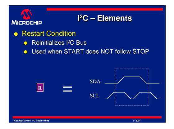
Next is the *Restart* condition. A restart condition indicates that a device would like to transmit more data, but does not wish to release the line. This is done when a start must be sent, but a stop has not occurred. It is also a convenient way to send a stop followed by a start right after each other. It prevents other devices from grabbing the bus between transfers.
