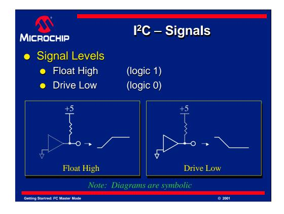
$I^2C$  lines can have only two possible electrical states. These states are known as "float high" and "drive low".  $I^2C$  works by having a pull-up resistor on the line and only devices pull the line low. If no device is pulling on the line, it will "float high". This is why pull-up resistors are important in  $I^2C$ .
