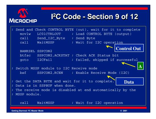
Its time now to send the control out byte. This tells the EEPROM to send data out to the PICmicro MCU. After we check for the ACK condition, it is time to receive the data.
