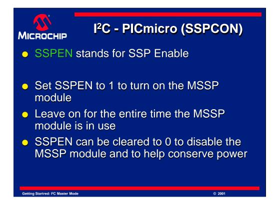
SSPEN is the "Synchronous Serial Port Enable" bit.
