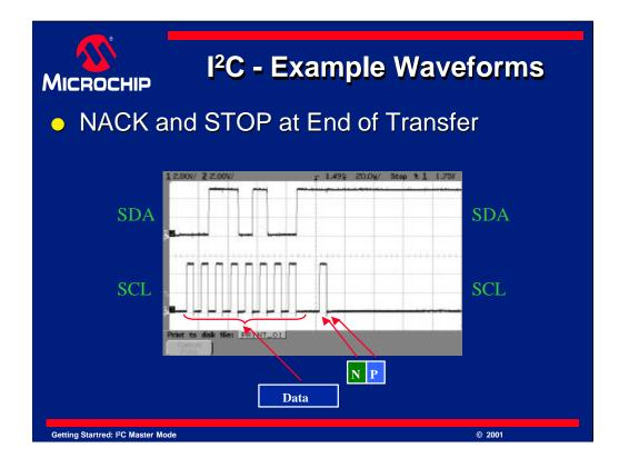
This slide has zoomed in on the last byte in the transfer. It contains the data that was retrieved from the EEPROM, the NACK sent by the PICmicro and the stop condition. Once these signals have finished, the bus is idle as there is no more data or conditions on the bus. This can be seen from the right of the stop condition. Once the stop condition completes, we have finished communicating with the EEPROM.
