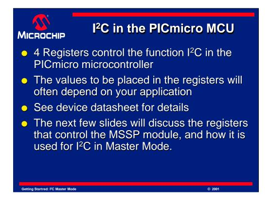
I2C on the PICmicro is controlled by 4 registers which we will look at in detail shortly. The values placed in these registers will control every aspect of the I<sup>2</sup>C communication. The device datasheet and reference manual will contain many details on using I<sup>2</sup>C and configuring these values, but we will give an introduction to them here. Note also that the MSSP module on a PICmicro device is capable of many different modes and configurations.
