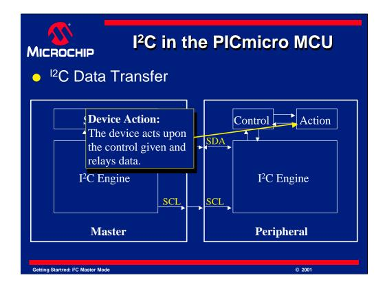
The device action block represents that once the  $I^2C$  request is decoded, it will either generate an action by the peripheral or it will generate data which is sent via  $I^2C$ .
