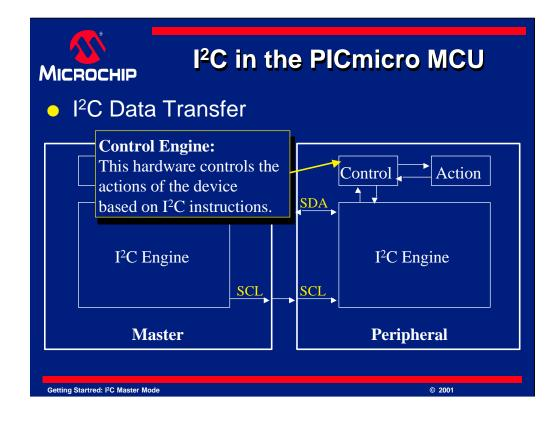
The peripheral will also contain a control engine of some kind. This engine will recognize valid  $I^2C$  commands and direct that the peripheral perform the desired action. It could be thought of as a kind of instruction decoder. This same block will also take the data generated from the action of the device and communicate this to the  $I^2C$  engine for transmission.
