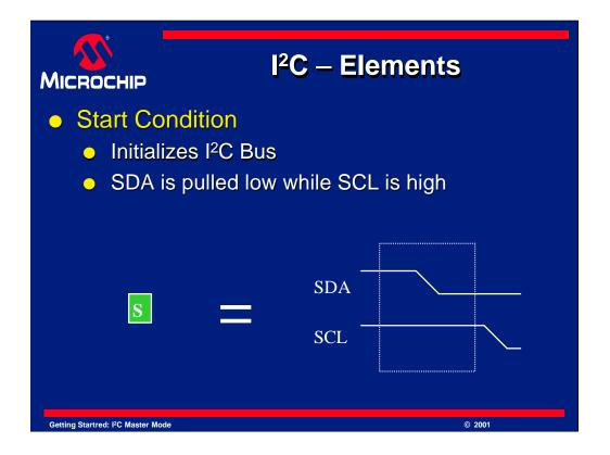
The first element we need to look at is the *Start* condition. A start condition indicates that a device would like to transfer data on the  $I^2C$  bus.
