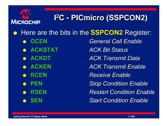
The SSPCON2 register is other register that controls the I<sup>2</sup>C engine on the PICmicro microcontroller.
