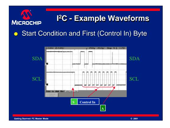
Here is a close up of a start condition, the control in byte and its ACK. You can clearly see the data now. After the start, SDA goes high, then low, then high again. Then it remains low until the spike. This translates into a data bit at each clock pulse. At the first SCL pulse, SDA is high, so this bit is a 1, then it goes low for the next pulse so this is a 0, and so on. You should be able to recognize the binary value of 1010 0000, or 0xA0 (hex).
