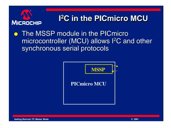
In the PICmicro, a module is used for the  $I^2C$  protocol. This module is named the MSSP module and allows SPI or  $I^2C$  to be implemented.
