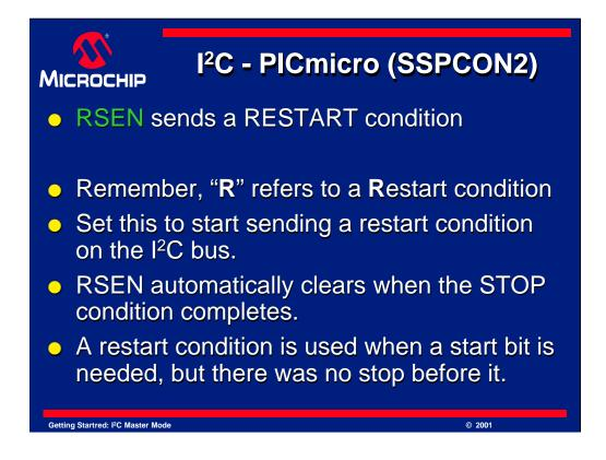
RSEN allows the user to send a restart condition on the I<sup>2</sup>C bus.
