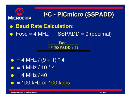
If Fosc were 4 MHz, and SSPADD were 9 (decimal), then lets calculate the I<sup>2</sup>C speed:
