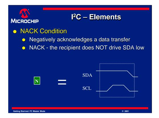
This is a *NACK* condition. Remember that a "ACK"'s or "NACK"s a byte of data.  $I^2C$  states that each byte MUST be answered with a NACK or ACK. If the device can not decide if it wants to ACK or NACK, then it will hold the clock line low until it makes up its mind. This action is known as "clock stretching" and is a feature of  $I^2C$  to give devices enough time to respond. We will look at this in more detail later.
