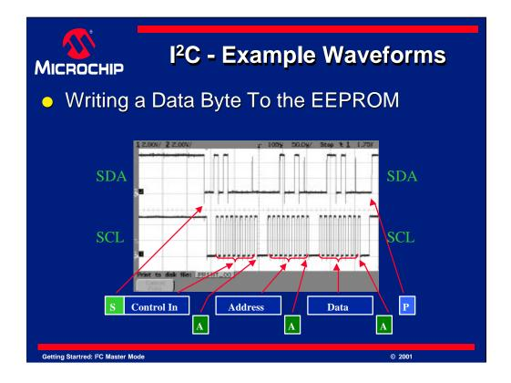
Here is a close-up of the writing to the EEPROM. The diagram points to the various conditions that make up the write transfer sequence. Note, even though the arrows appear to only point to the SDA or SCL signals, both the SDA *and* SCL are part of each condition. For example, data is not data unless there is a clock for it, and a Start condition is made up of the timing of *both* SDA and SCL.
