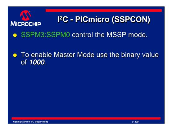
SSPM3:SSPM0 are 4 bits that yield 16 different Synchronous Serial Port modes.
