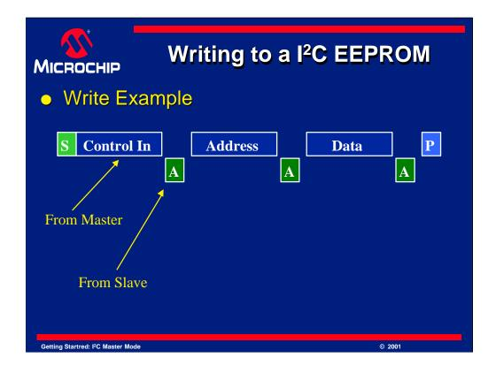
If we put these elements together, we can produce useful I2C transfers. The aim of this presentation is to communicate with a serial  $I^2C$  EEPROM. Here is an example transfer of *writing* to a small EEPROM.
