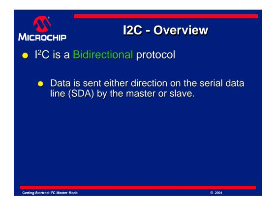
$I^2C$  is a Bi-directional protocol. Data can flow in any direction on the  $I^2C$  bus, but when it flows is controlled by the master device.
