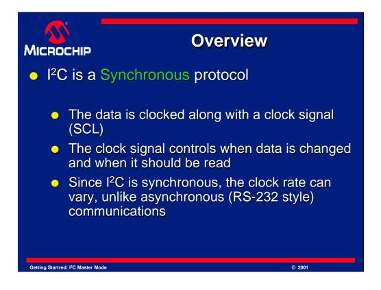
$I^2C$  is a synchronous protocol that allows a master device to initiate communication with a slave device. Data is exchanged between these devices.
