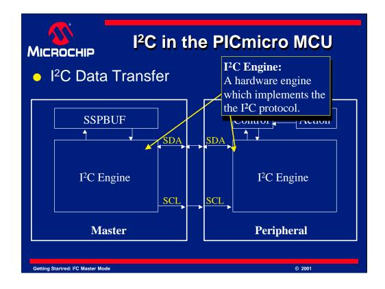
The I<sup>2</sup>C engine sends data out on the I<sup>2</sup>C bus using the Clock (SCL) and Data (SDA) lines for communication. The I<sup>2</sup>C engine on the PICmicro device contains many registers which configure it as well as control its operation. The user has full access to these registers and we will look at them later in this presentation.
