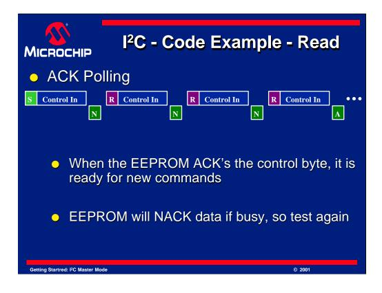
There is one problem with the approach we just discussed. If the EEPROM is busy, it will NACK the next command. This NACK will occur after we send the control byte. See the diagram here. If it is still busy, it will NACK again. If one were to keep sending a control byte, one could discover exactly when the EEPROM was ready. Doing this allows the fastest access time and is called "ACK Polling".
