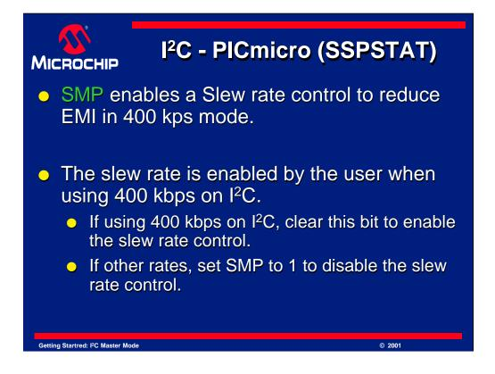
SMP enables the slew rate control of the MSSP module.
