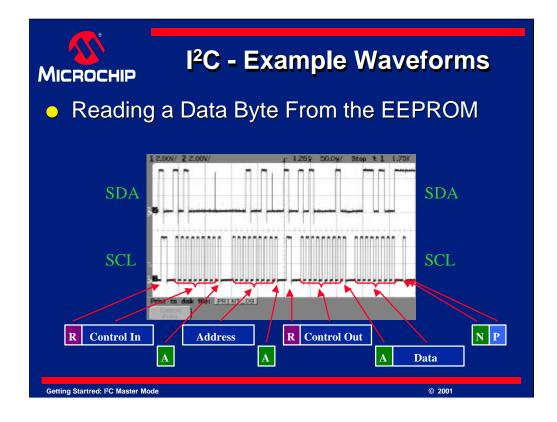
Here is a look at our EEPROM read waveform. Shown here is the first control byte that is ACKed by the EEPROM. None of the ACK polling is shown here. You can see the Control in byte, which has the value of 0xA0 (hex). You can also see the address byte and data byte. Remember we wrote 0x34 (hex) to address 0x12 (hex).
