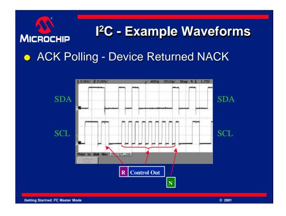
Here we have zoomed in on one loop. You can clearly see the restart, the control out byte, and the NACK. The NACK is now easy to see. Notice that one the 9th clock pulse the SDA line goes high. This indicates the bit is a 1, which signifies a NACK response.
