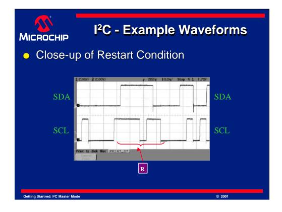
Here is a closer look at the same restart condition. You can now clearly see the stop and start condition contained within it. Remember, a stop condition is a release of the SCL line followed by a release of the SDA line. A start condition is when SDA is pulled low, followed by SCL. Restart conditions may sometimes look different from each other, but they must contain a stop followed by a start condition by definition.
