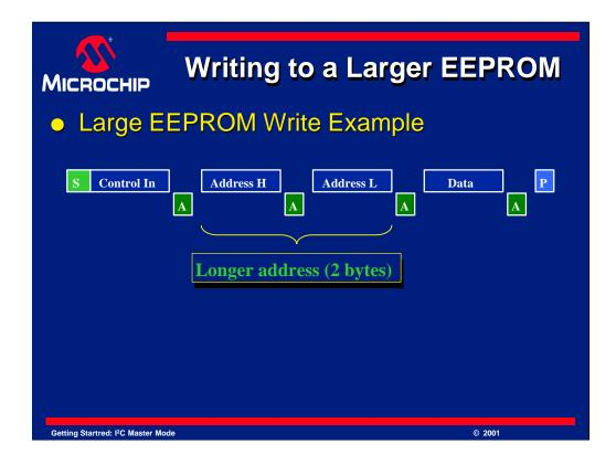
Writing to a large EEPROM is not very different from a small one. The only difference is there are now *two* address bytes instead of one. As you would expect, each byte must be "ACK'ed" as well.
