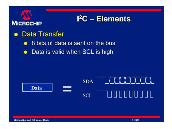
Let's now discuss the data transfer element. The data block represents the transfer of 8 bits of information. The data is sent on the SDA line and SCL produces a clock. The clock can be aligned with the data to indicate whether each bit is a "1" or a "0".
