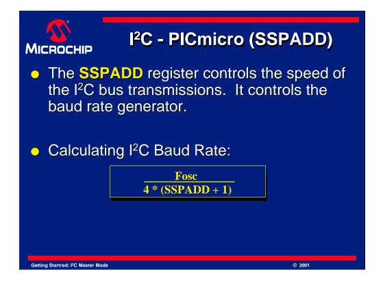
The the last register to be discussed that controls I<sup>2</sup>C is the SSPADD register. SSPADD stands for "Synchronous Serial Port ADDress", but in master mode this register has a different function. This register controls the speed of the I<sup>2</sup>C bus. The I<sup>2</sup>C bus speed is a calculation based on Fosc, which is the clock speed of the microcontroller, and the value loaded into SSPADD.
