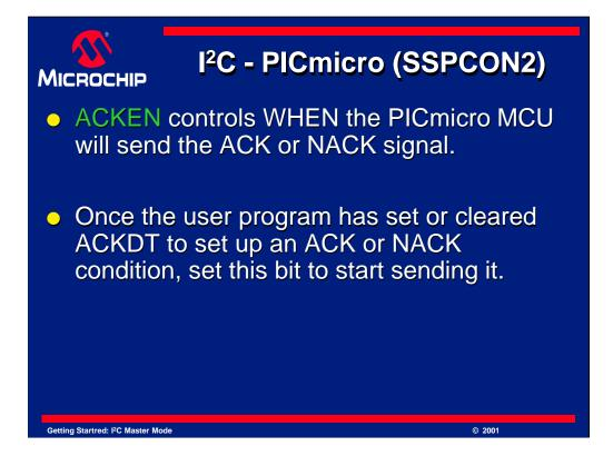
ACKEN controls exactly *when* the acknowledge bit is sent. Regardless of the state of ACKDT, it is not sent *until* ACKEN is set. This allows one to set up the desired acknowledge bit to be sent, then send it when ready.
