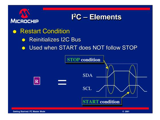
Here we can clearly see that the signaling used for a restart can be seen to be nothing more than a stop condition quickly followed by a start condition. Remember that a stop condition is when SDA goes high while SCL is high. A start condition is when SDA is pulled low while SCL is high.
