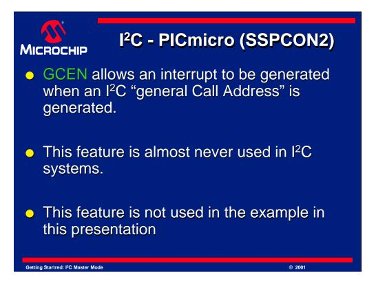
GCEN is a feature of  $I^2C$  that allows the MSSP module to be backward compatible with older and/or slower systems. It is almost never used in an  $I^2C$  system and is not used for our example. For more information on the "General Call" feature of  $I^2C$ , consult the  $I^2C$  specification.
