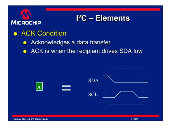
Lastly we will discuss the *ACK* and *NACK* condition. A device can "ACK" or acknowledge a transfer of each byte by bringing the SDA line low during the 9th clock pulse of SCL.
