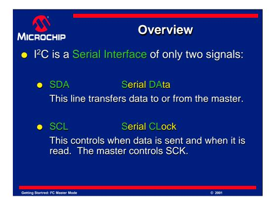
$I^2C$  is a Serial Interface and uses only the following two signals to serially exchange data with another device:
