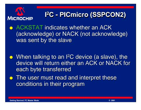
The ACKSTAT bit is set when an ACK or NACK has been received from the peripheral device. Remember, the peripheral must acknowledge all data bytes, and this is done by sending an ACK or NACK condition. This bit can be polled or tested to determine if an ACK or NACK condition has occurred. Its usage will be shown in our example program, which we will see later in this presentation.
