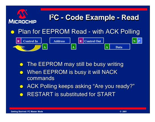
Notice in this diagram the start condition has been changed to a restart condition. This is done because a restart is simply a stop followed by a start condition. So, even if we just had a stop before the restart, we get two stops, followed by a start. Two stop conditions in a row is not a problem and perfectly legal in I<sup>2</sup>C. So, the start has been replaced with a restart.
