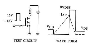
$$\begin{split} R_G = 25~\Omega \\ V_{DD} = 90~V,~L = 16.8~mH \end{split} \label{eq:RG}$$
