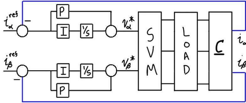
**Figure 5.25 – Stationary current control.**
