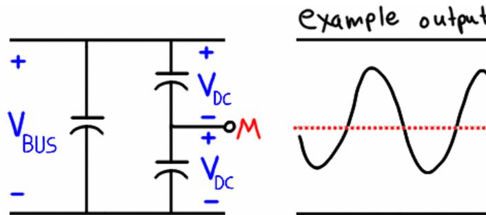
Figure 4.2 – Definitions of DC bus midpoint and voltage magnitudes.
