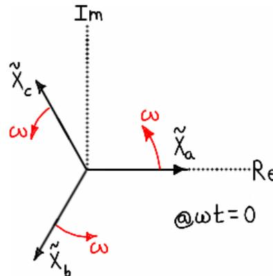
Figure 3.18 – Positive sequence phasor orientation.
