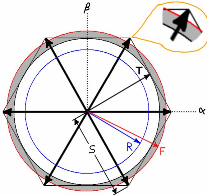
**Figure 4.34 – SVM overmodulation region: locus of fundamental SV.**
