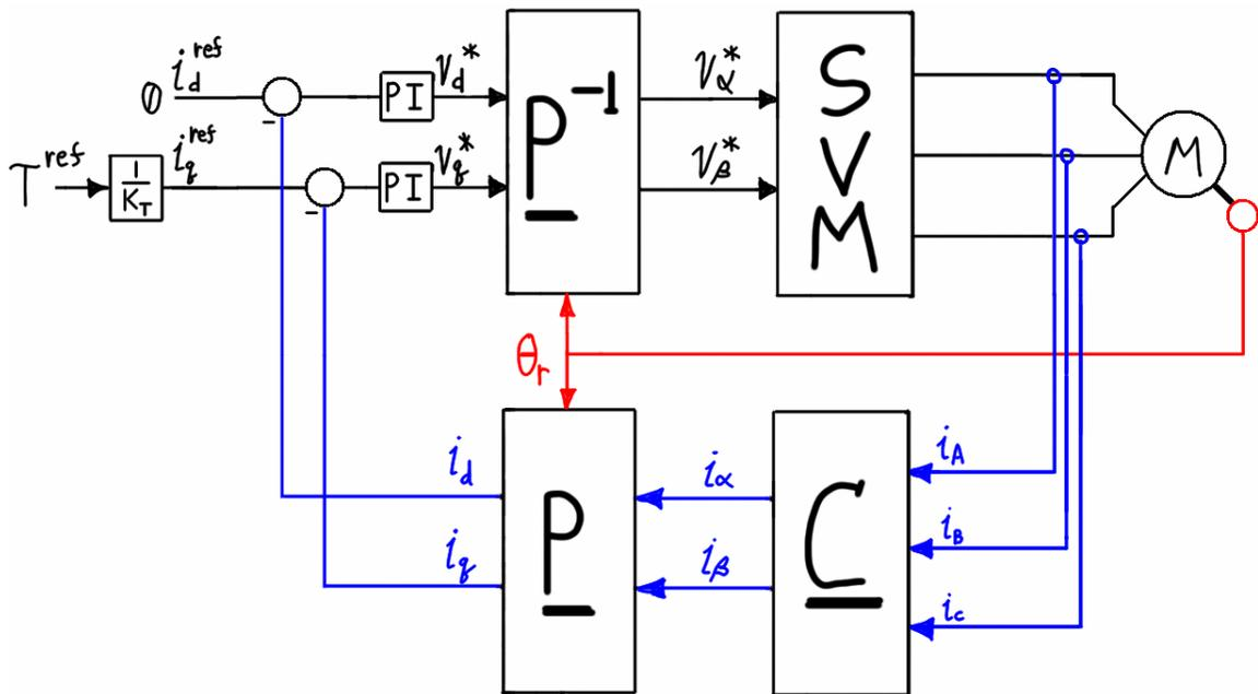
Figure 5.14 – Field oriented control with SVM.
