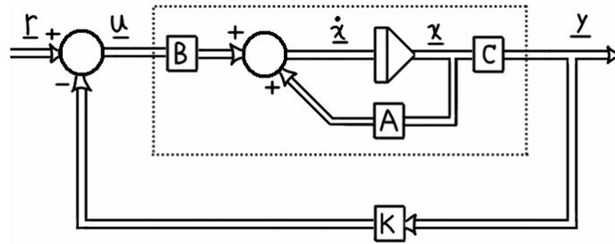
**Figure 6.4 – Output feedback controller.**
