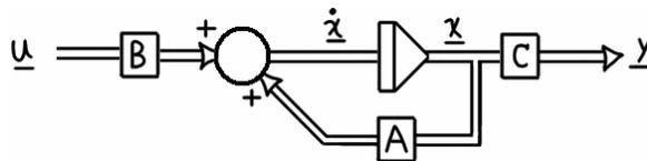
**Figure 6.3 – State-space representation of linear system.**
