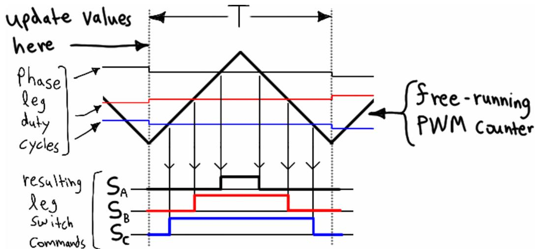
**Figure 4.41 – Generating leg switch commands.**
