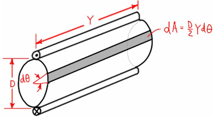
Figure C.13 – Single-turn full-pitch winding.
