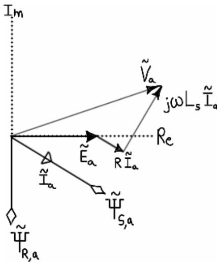
**Figure 3.22 – Time relationships between electrical and magnetic quantities.**
