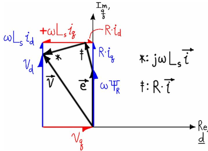
Figure 3.43 – Steady-state SV diagram in rotor frame; voltage and EMFs.
