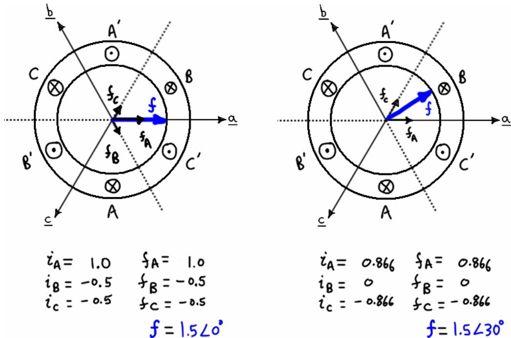
Figure 3.11 – Instantaneous values of component and total MMFs; (c.f. Figure 3.7, Figure 3.8).
