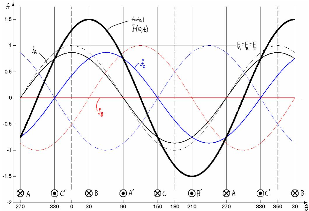
**Figure 3.8 – Developed view at thirty electrical degrees.**
