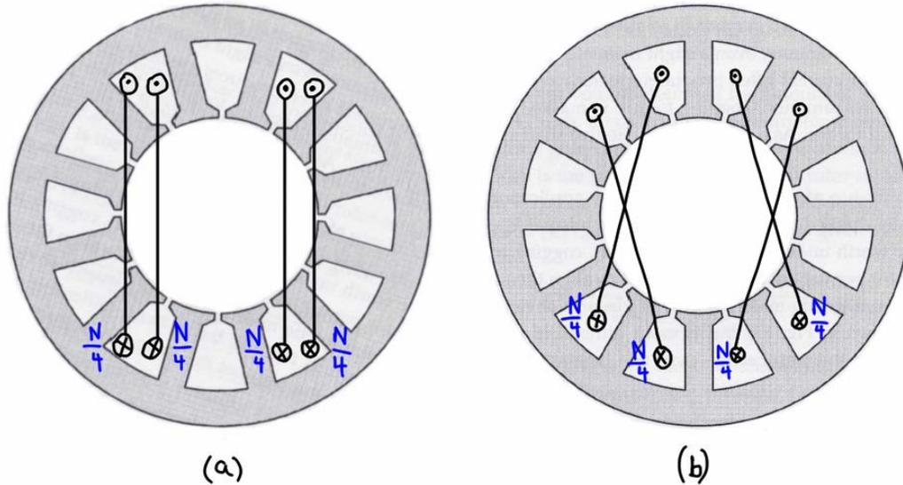
**Figure C.6 –Short-pitched windings: (a) concentrated; (b) distributed.**
