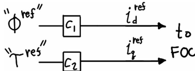
Figure 5.22 – "Torque" and "flux" control.
