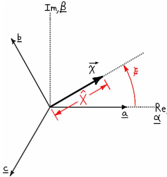
**Figure 3.29 – Arbitrary space vector in the complex/ $\alpha\beta$  plane.**
