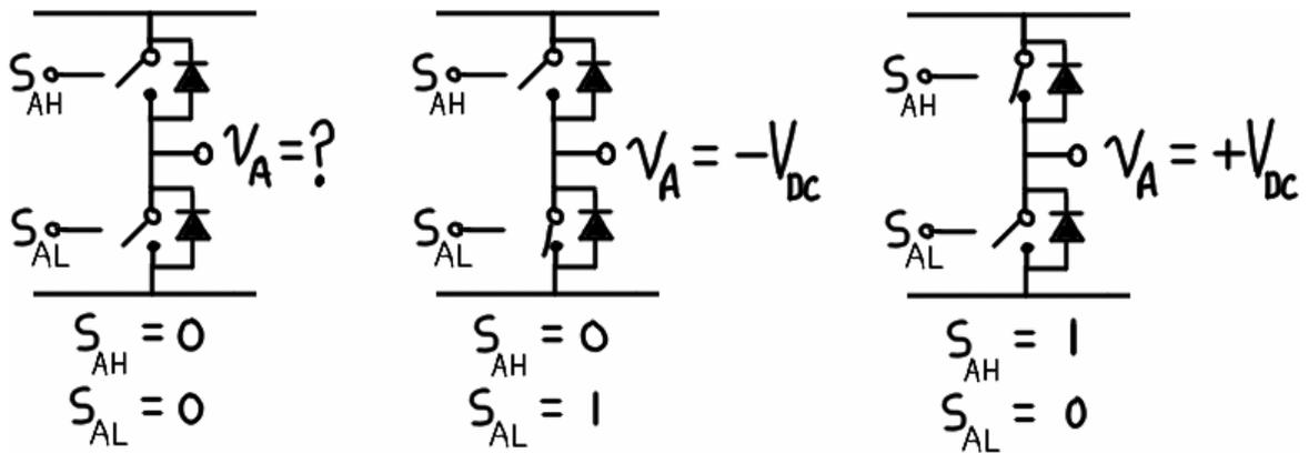
Figure 4.5 – Leg states for 120° inverter.
