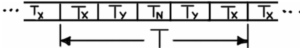
Figure 4.36 – One period in an improved switching scheme.
