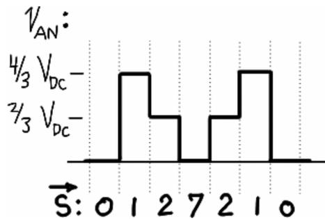
Figure 4.39 – Phase-A line-neutral voltage; commanded SV in sextant  $s_{12}$ .
