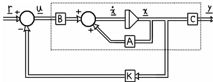
**Figure 6.5 – Full state feedback controller.**
