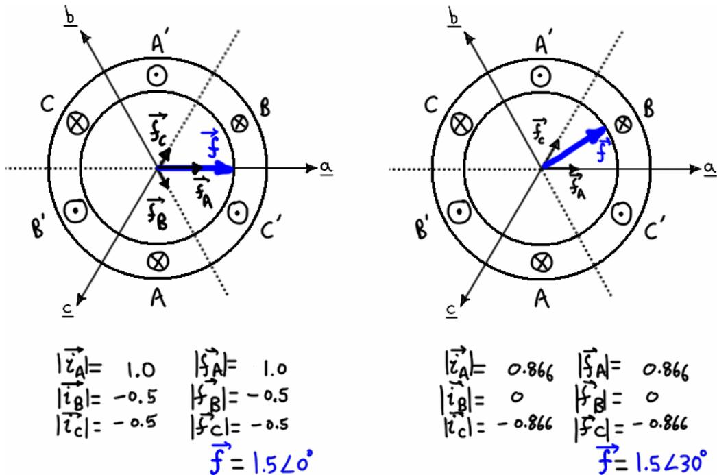
Figure 3.25 – Instantaneous values of component and total MMF space vectors; (c.f. Figure 3.11).
