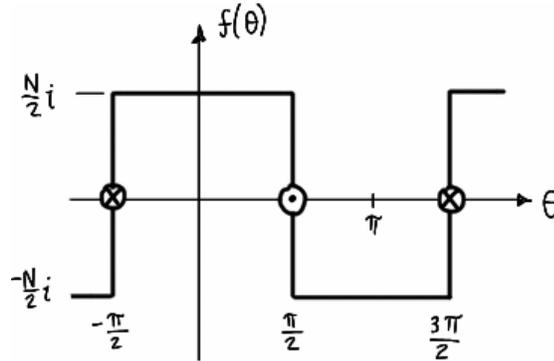
Figure C.9 – MMF of CFP winding.
