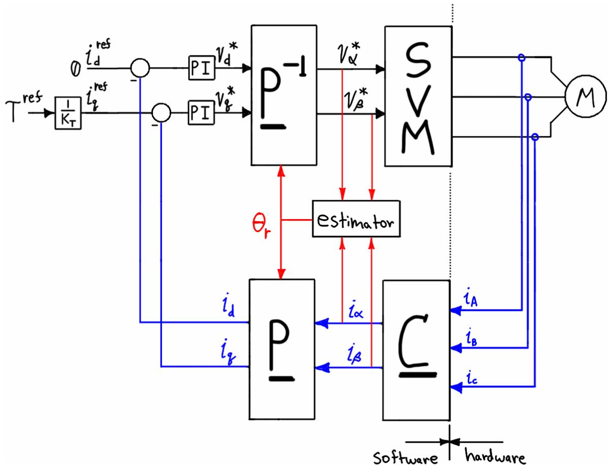
Figure 6.1 – General sensorless FOC structure.
