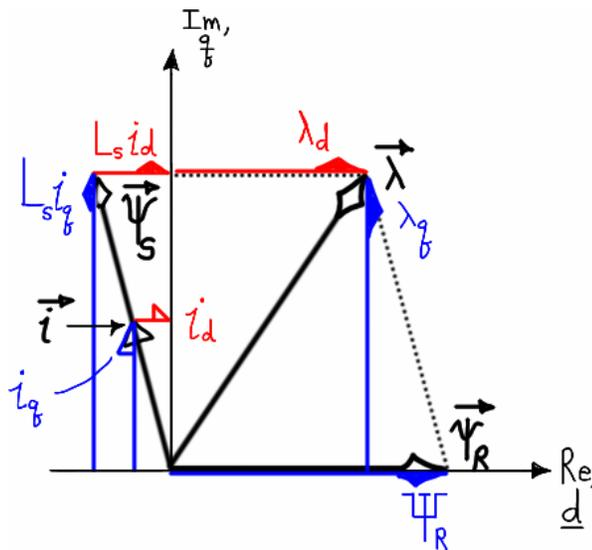
Figure 3.44 – Steady-state SV diagram in rotor frame; current and flux linkages.
