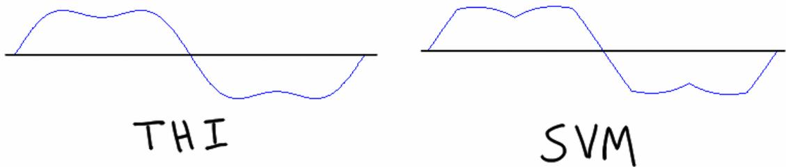
**Figure 4.43 – Average pole voltages for THI and SVM inverter.**
