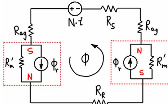
Figure 2.14 – Magnetic circuit of Figure 2.12.
