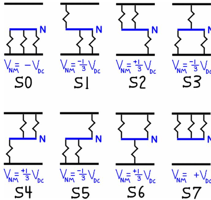
Figure 4.21 – Inverter states and neutral voltages.
