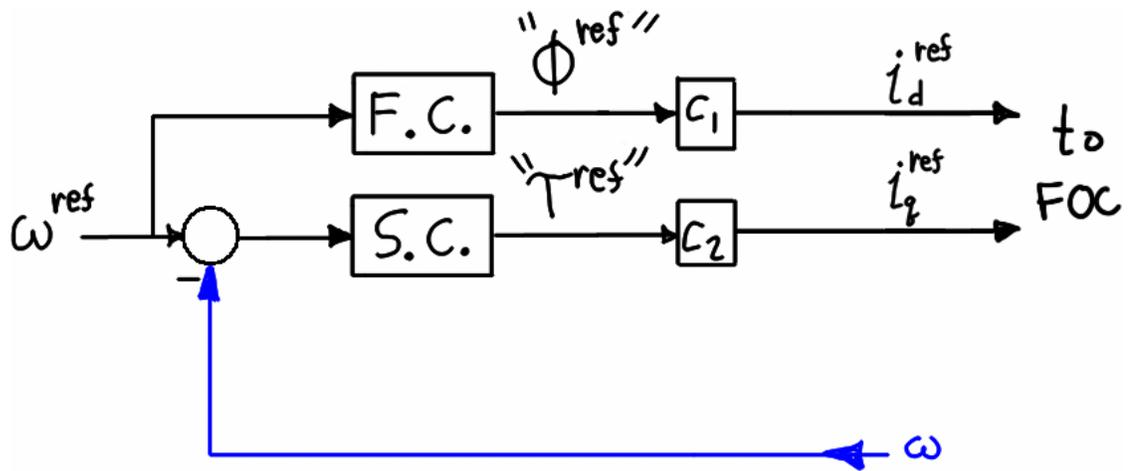
Figure 5.23 – Field weakening controller.
