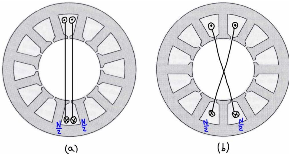
**Figure C.5 – Full-pitch windings: (a) concentrated; (b) distributed.**
