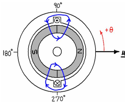
**Figure 2.12 – Section view of a general brushless PM motor.**
