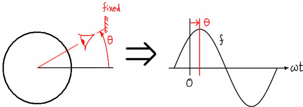
**Figure 3.10 – Observing MMF value at fixed position.**
