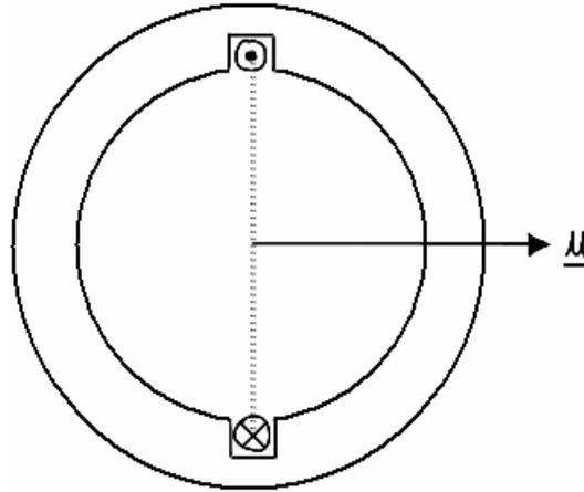
**Figure C.2 – Concentrated full-pitch (CFP) winding.**
