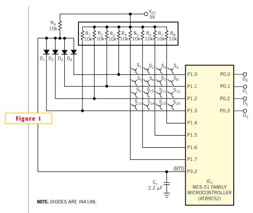
Adding an interrupt-driven keypad to an MCS-51 family microcontroller requires only a few components.
