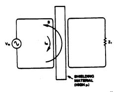
Magnetic shielding is not as easily accomplished as electrostatic shielding, but may be done at HF with a simple conducting screen, and at LF and DC with a screen of high permeability material such as Mu-metal.
