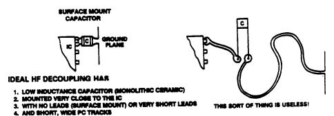
IT MAY BE SHUNTED WITH A TANTALUM BEAD ELECTROLYTIC TO PROVIDE GOOD LF DECOUPLING AS WELL
