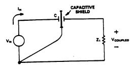
EQUIVALENT CIRCUIT ILLUSTRATES HOW A CAPACITIVE SHIELD CAUSES THE NOISE CURRENTS TO RETURN TO THEIR SOURCE WITHOUT FLOWING THROUGH Z<sub>1</sub>
