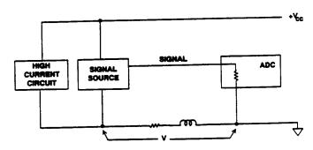
V = VOLTAGE DUE TO SIGNAL CURRENT AND CURRENT FROM HIGH CURRENT CIRCUIT FLOWING IN GROUND IMPEDANCE
