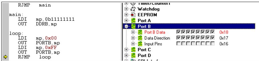
The screenshot shows the AVR simulator interface. On the left, the assembly code is displayed:
