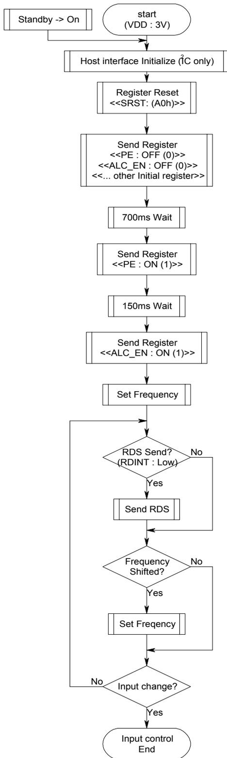
For communication with I<sup>2</sup>C, reset the host interface right after the power activation to ensure the communication.
