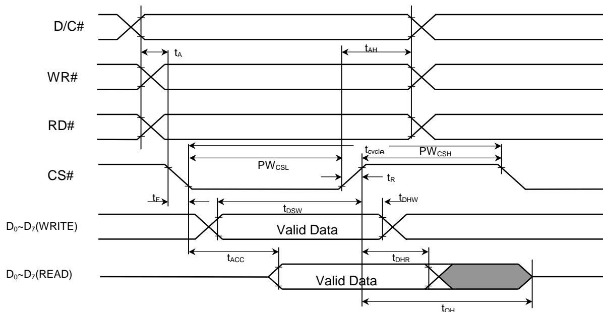
**Figure 11 - 8080-series MPU Parallel Interface Characteristics**
