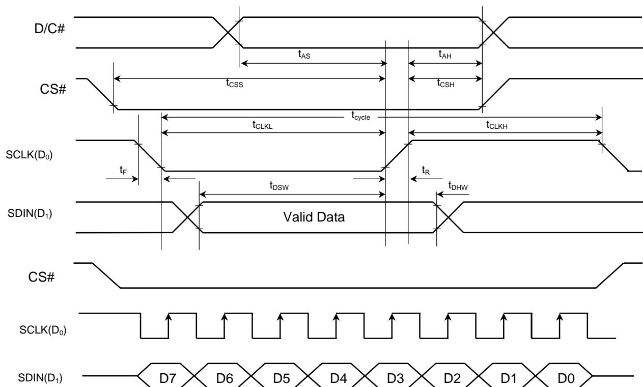
**Figure 12 - Serial Interface Characteristics**
