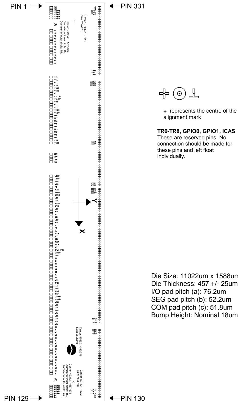
Figure 2 - SSD0323Z Gold bump die pad assignment
