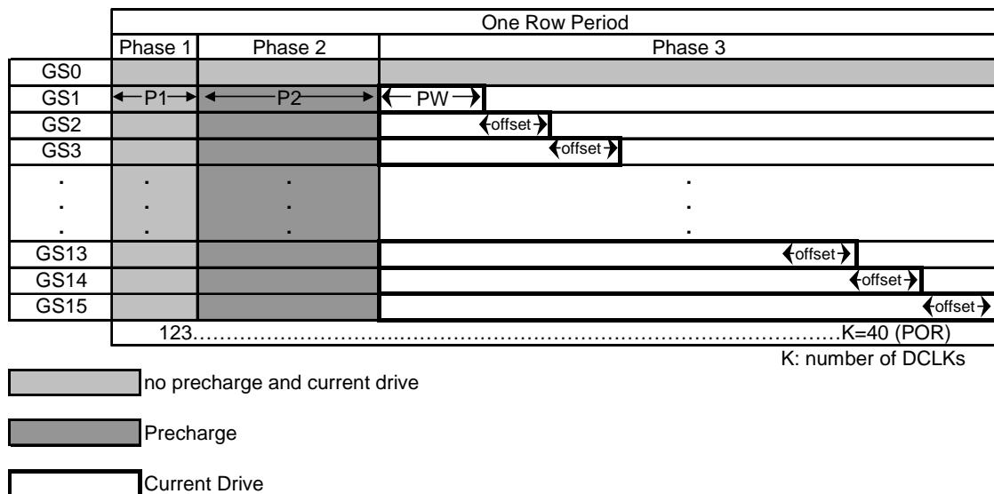
Figure 5 - Gray scale pulse width set diagram
