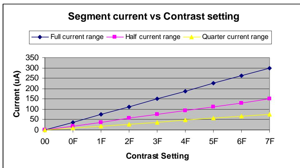
Figure 6 - Segment current vs Contrast setting
