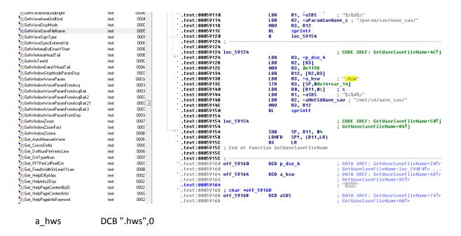
once the file extension is .hsw and another time it is .hws – this is preventing the save/reload from USB to work properly and even sometimes crashing DSO.
