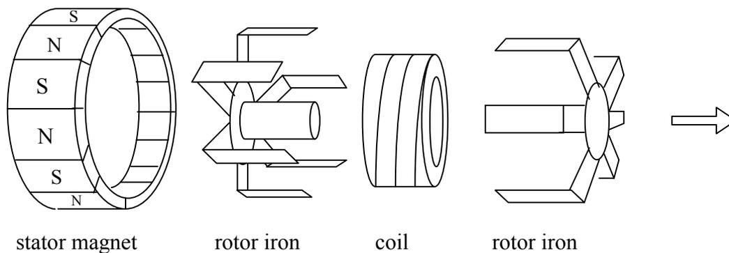
Fig.3: Assembly of a hub dynamo
