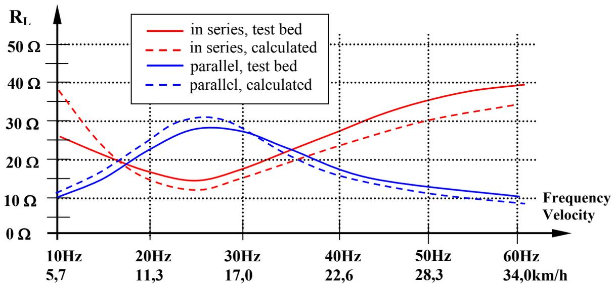
Fig.7: Optimal load resistance versus frequency according to test bed and calculation
