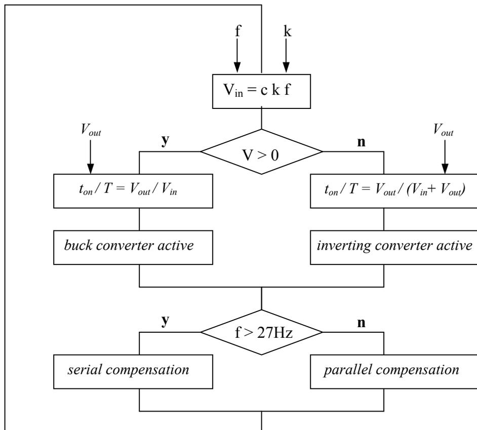
Fig.11: Converter control flow chart
