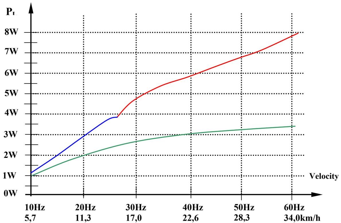
Fig.12: Power versus velocity for conventional case (green) and our proposed solution (blue, red)
