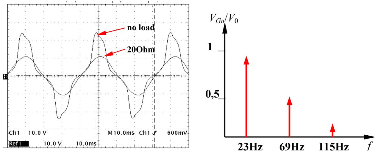
Fig.5: Voltage versus time without load and with 20 Ohm load, Time function and spectrum
