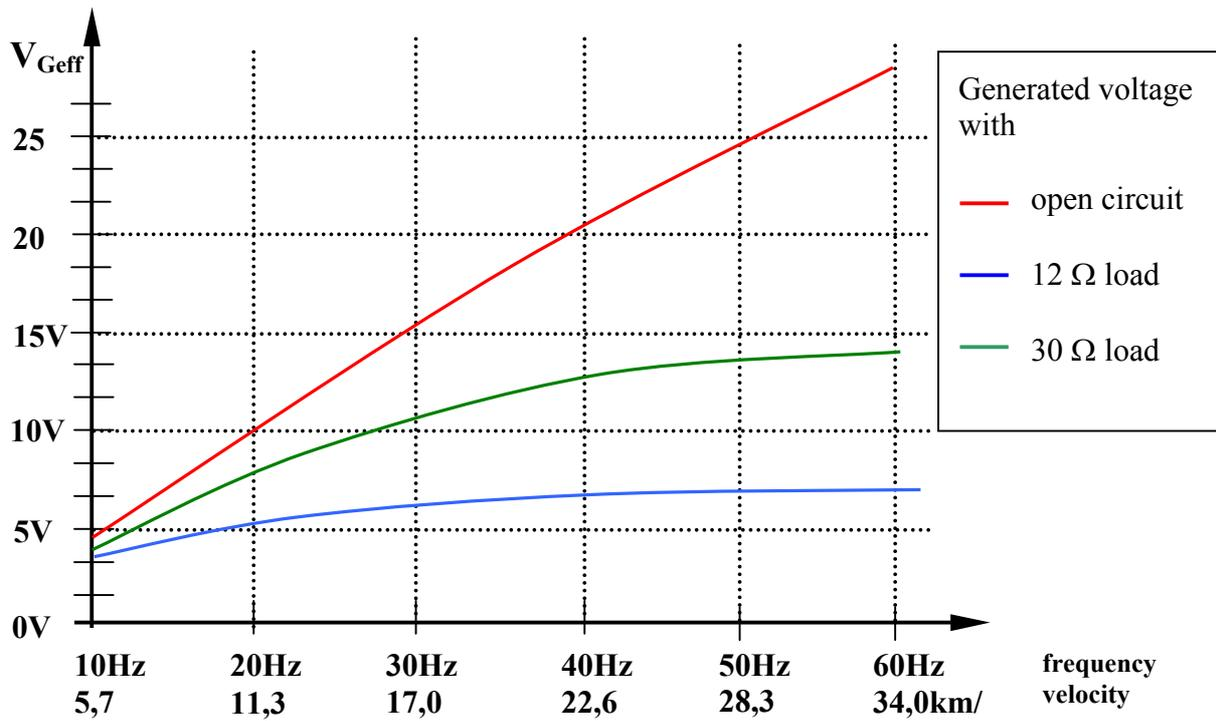
Fig.4: Generator output voltage versus frequency for different loads
