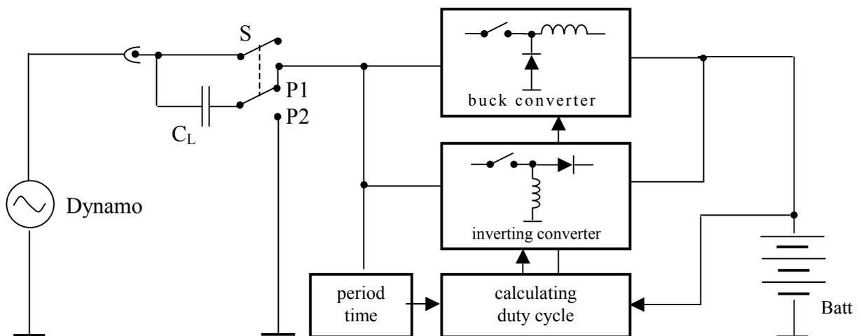
Fig 10: Converter block scheme with dynamo and battery
