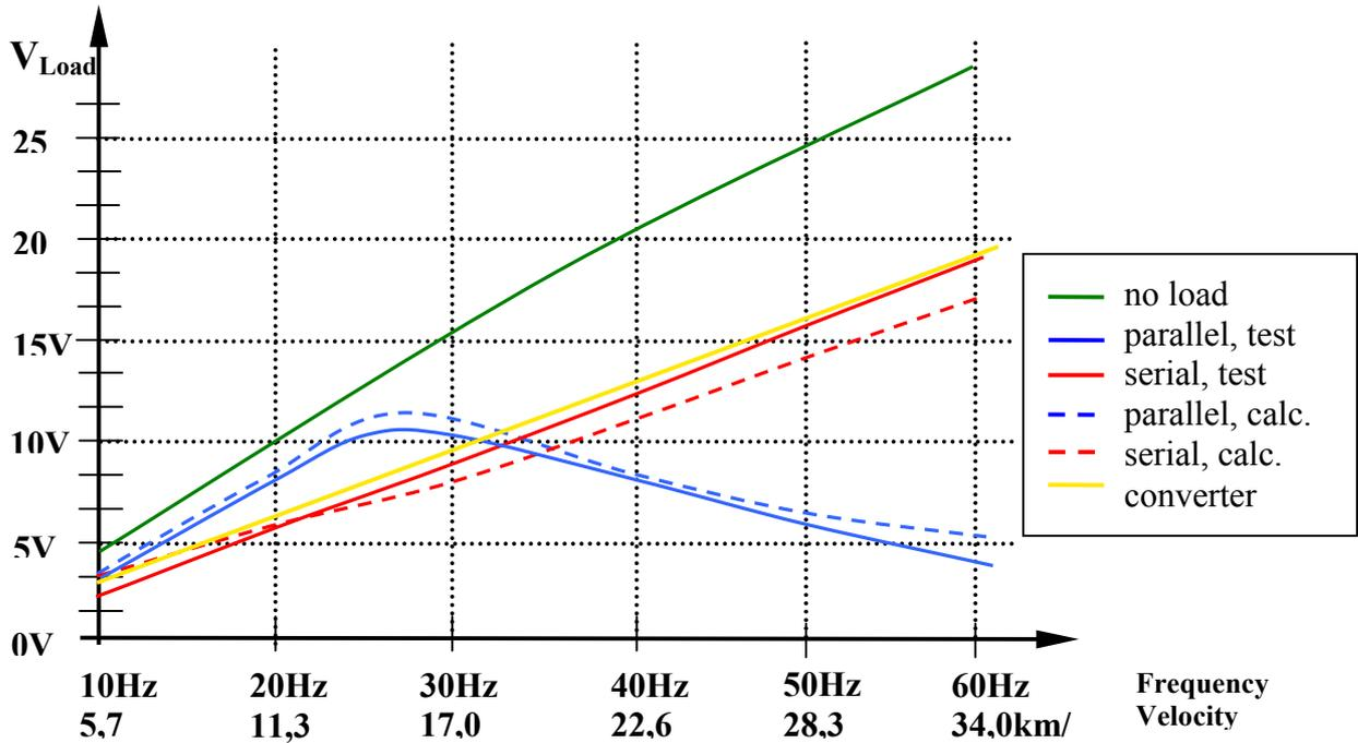
Fig.9: Voltage over optimal  $R_L$  versus frequency according to test bed and calculation
