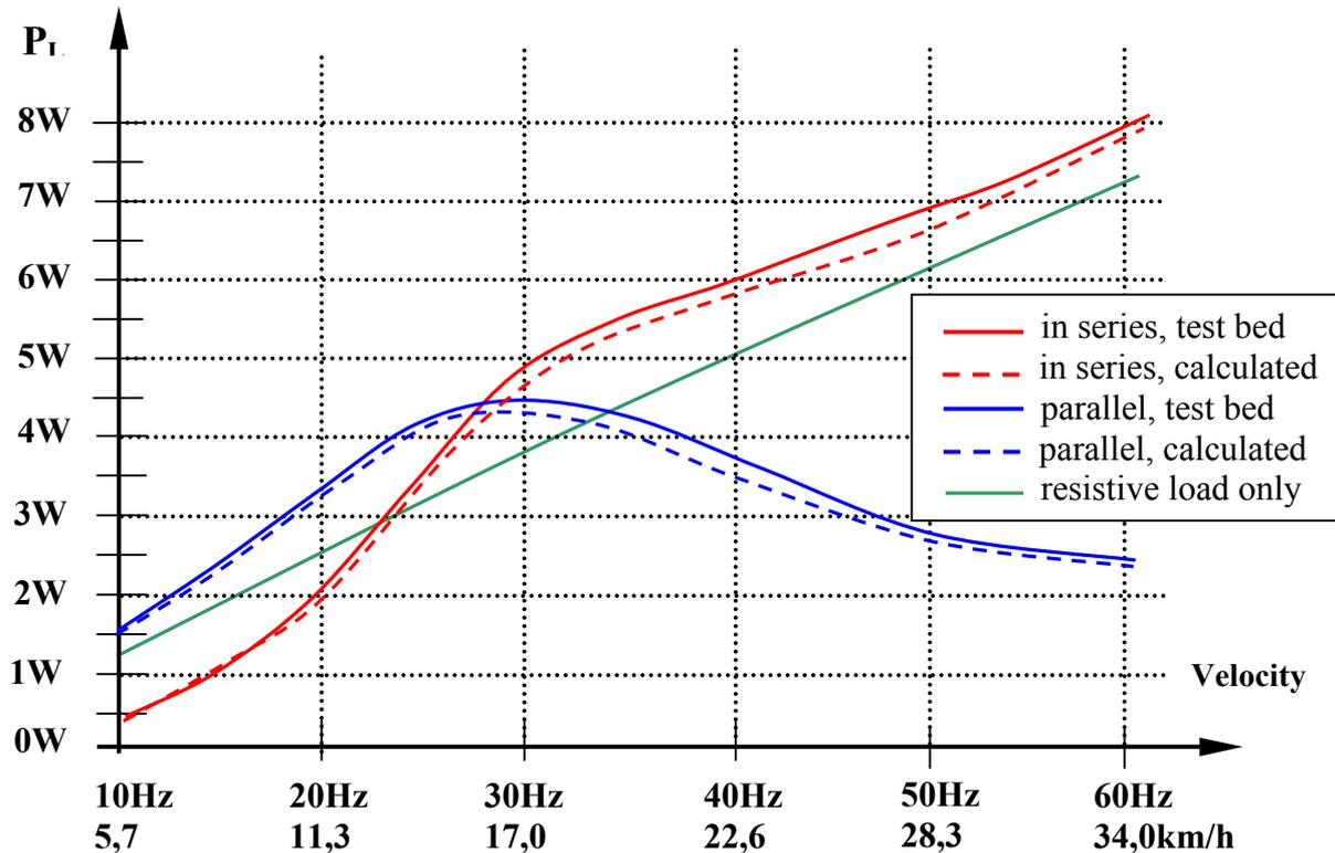
Fig.8: Output power versus frequency according to test bed and calculation
