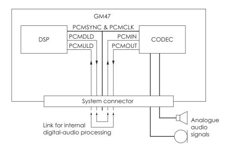
Figure 2.4 Pin connections to digital audio
