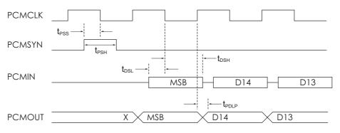
Figure 2.7 PCM Timing Diagram
