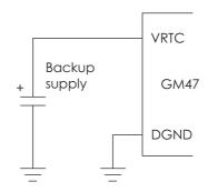
Figure 2.10 RTC connections
