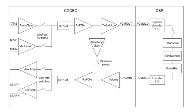
Figure 4.1 Audio diagram of the CODEC
