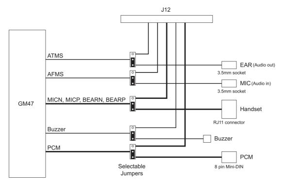
Figure 1.4 Audio signals, connection and routing
