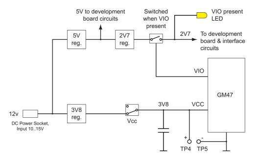
Figure 1.2 Power supply connection and the on-board voltages
