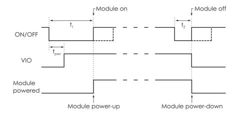
Figure 2.2 ON/OFF timing and VIO performance
