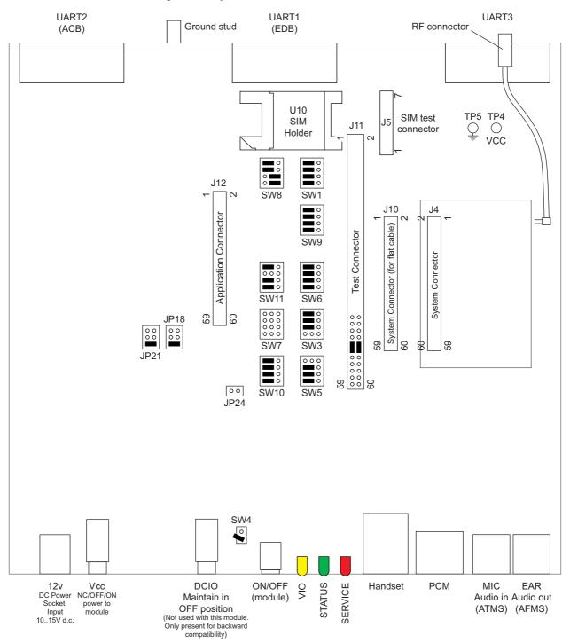
Figure 2.3 Developer's board overlay
