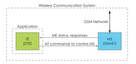
Figure 2.1 Main Blocks in a Wireless System
