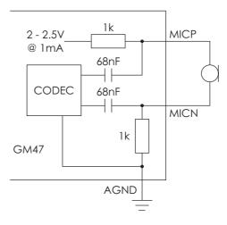
Figure 2.3 Microphone connections to the module
