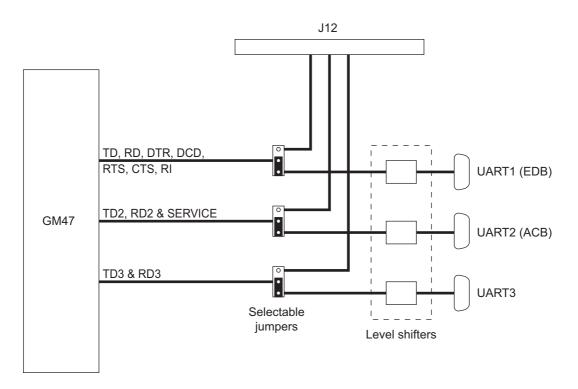
Figure 1.5 Comms signals, connection and routing
