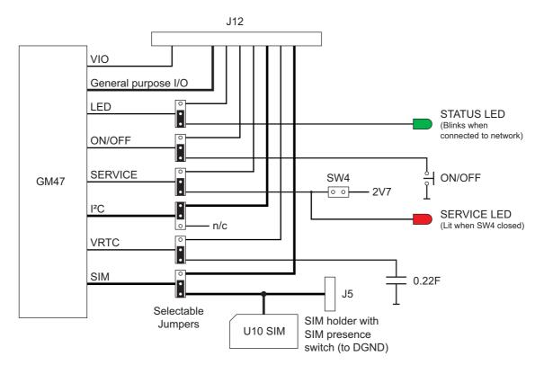
Figure 1.3 Miscellaneous signals, connection and routing
