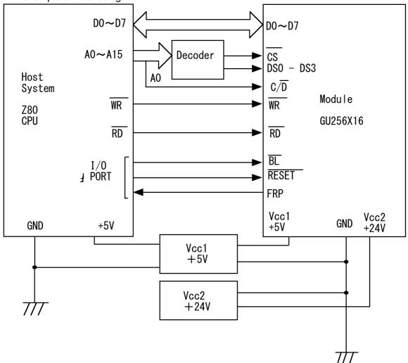
Since data execution time of the module is 2u Sec.(MAX.), there are no BUSY or READY output. Therefore more than 2u Sec. time period is required between module access.
