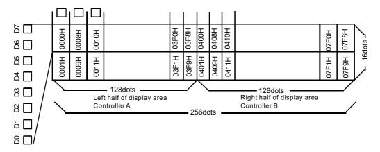
As shown the above, the display address is incremented 8 bytes horizontally. When display start address is changed, the display address adds the display start address and the above address.
