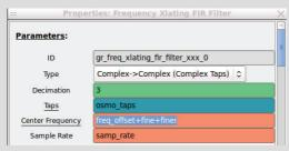
I also blindly copied the RF power display, a toggle for saving the audio files out to disk, and a  $+900 \rm khz$  tuning slider from other receivers. I added a second 'fine' tune  $+50 \rm Khz$ . This is done by setting the frequency of the Xlating FIR filter to,
