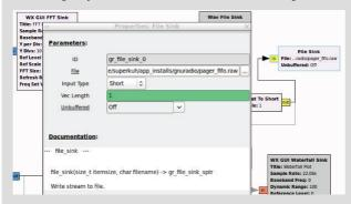
In my personal copy of dekar's pager\_fifo the file and audio sinks are enabled while the waterfall, wav, and other sinks are disabled. To enable the disabled (grey) block select them and press 'e' ('d to disable). The audio sink is set to pulseaudio ("pulse").
