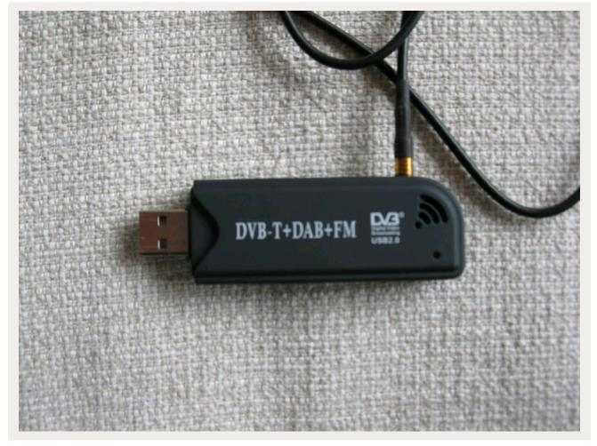
It was recently discovered that several cheap DVB-T usb dongles could be configured to be used as cheap ham radio receivers.
