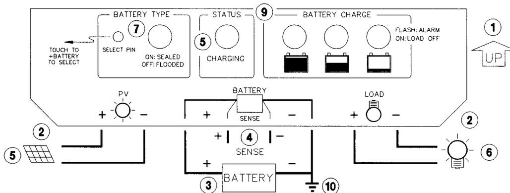
1. Mount the ProStar to a vertical surface. Allow space above and below the controller for air flow. The heatsink **MUST** be in a vertical (up & down) position.
