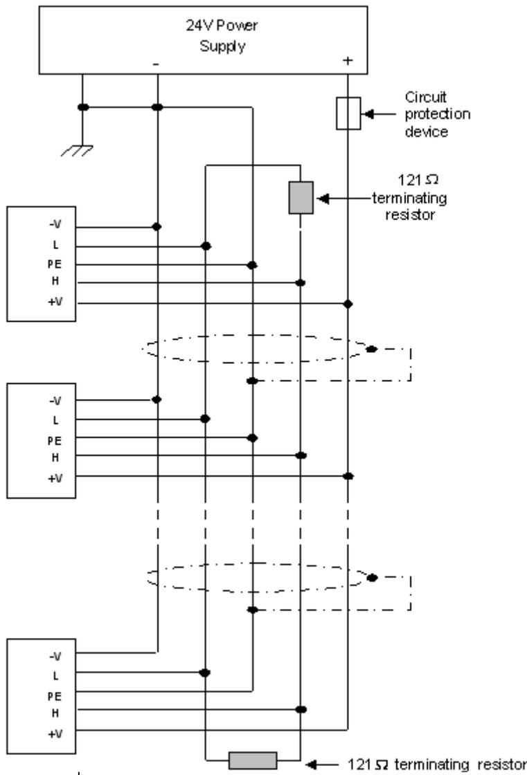
**Note •** Unitronics' CANbus control network is run by a **separate** isolated power supply that is **not** part of the network power supply.
