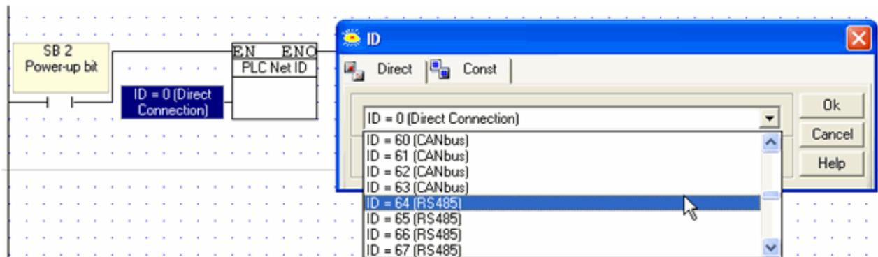
**Notes •** When the function is activated, the ID is written into the PLC. If the value is supplied via Indirect Vector, note that simply storing a value into the vector will not rewrite the ID. To rewrite the ID, the value must first be stored in the appropriate vector, and then the function must be activated.
