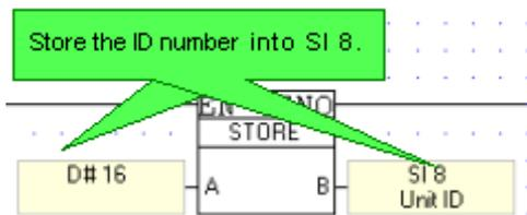
Linking a register value allows you to enable an end-user to enter an Unit ID number via the HMI panel. You can create a Display for this purpose as shown below.
