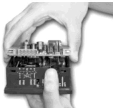
5. Locate the jumpers shown in the figure to the left, then change the jumper settings as required.
