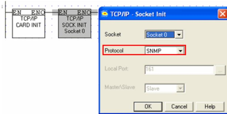
This enables any SNMP manager to access operand values in the Vision via UDP, port 161. Vision supports the following SNMPv1 commands, sent to the PLC from the network:
