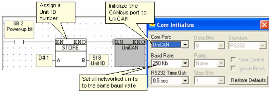
**Note •** Baud Rate is a function of cable length, as described in CANbus Hardware Specifications.
