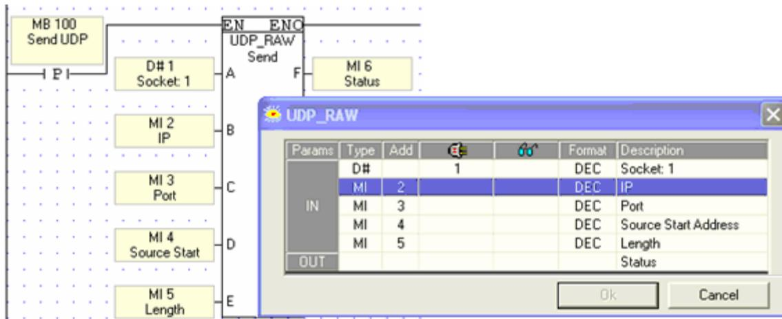
**Note •** Use a Send condition; do not place it directly on the left Ladder rail.
