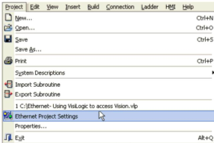
2. Open the IP Address Selector in order to enter the IP of the PLC s in the project.
