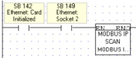
**TCP: controller-to-controller communication**
