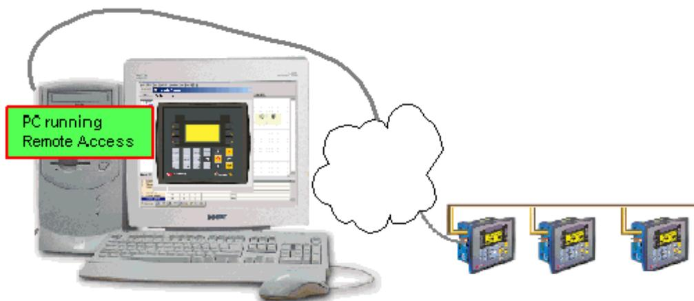
**Note •** In addition to using VisiLogic to access a remote Vision, Unitronics provides a stand-alone utility called Remote Access. This utility can
