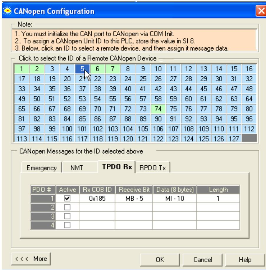
Send PDO RTR is a 'read' request, where the PLC requests data from the remote node. When the Configuration above runs with a Send PDO RTR as shown below, PDO message 1 is activated; 1 byte will be read from Node 5 into MI 10 in the PLC, and the Receive Bit for that message will turn ON.
