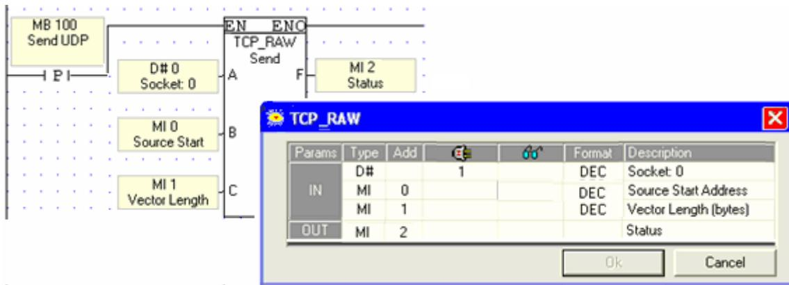
**Note** | Use a Send condition; do not place it directly on the left Ladder rail.
