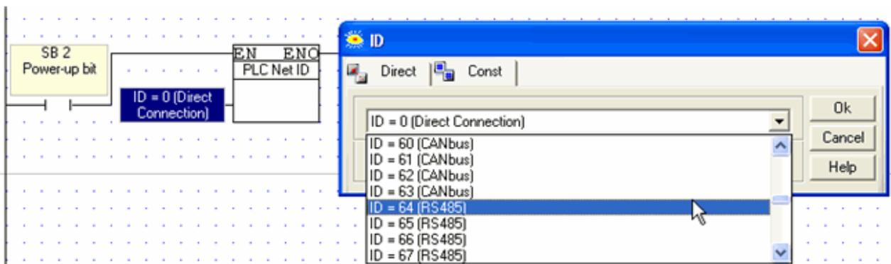
**Notes •** When the function is activated, the ID is written into the PLC. If the value is supplied via Indirect Vector, note that simply storing a value into the vector will not rewrite the ID. To rewrite the ID, the value must first be stored in the appropriate vector, and then the function must be activated.
