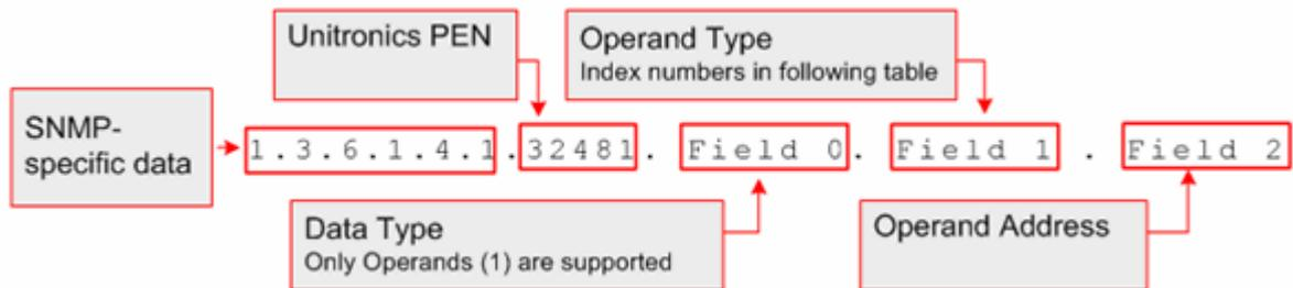
The table below shows the index numbers for operand types in Unitronics' controllers.
