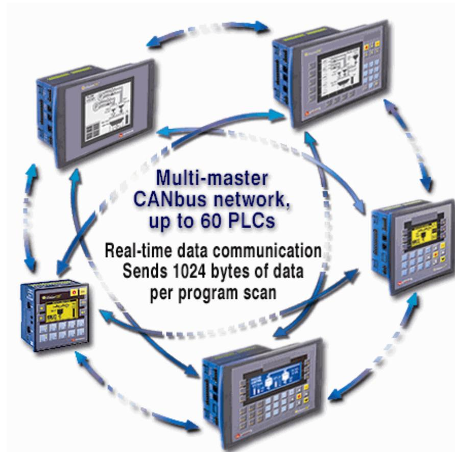
When PLCs are connected to the CANbus network and their CANbus ports initialized to UniCAN, you can use the UniCAN functions, located on the Communications menu, to transfer data between units or check a unit's status.
