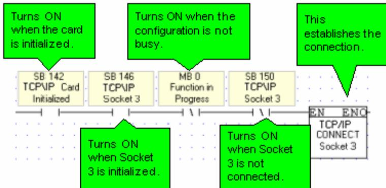
**Note •** It is recommended that there be a time elapse of a few seconds after the Ethernet Card Initialization and before activating Socket Connect. A timer may be used for this purpose.
