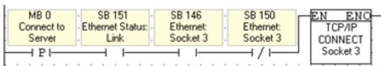
**Note •** It is recommended that you include a time elapse of a few seconds after the Ethernet Card initializes and before activating Socket Connect. A timer may be used for this purpose.
