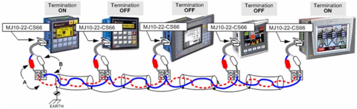
Note that, in the case of older V2xxx models comprising a third RJ45 COM port, a MJ10-22-CS65 connector is required.
