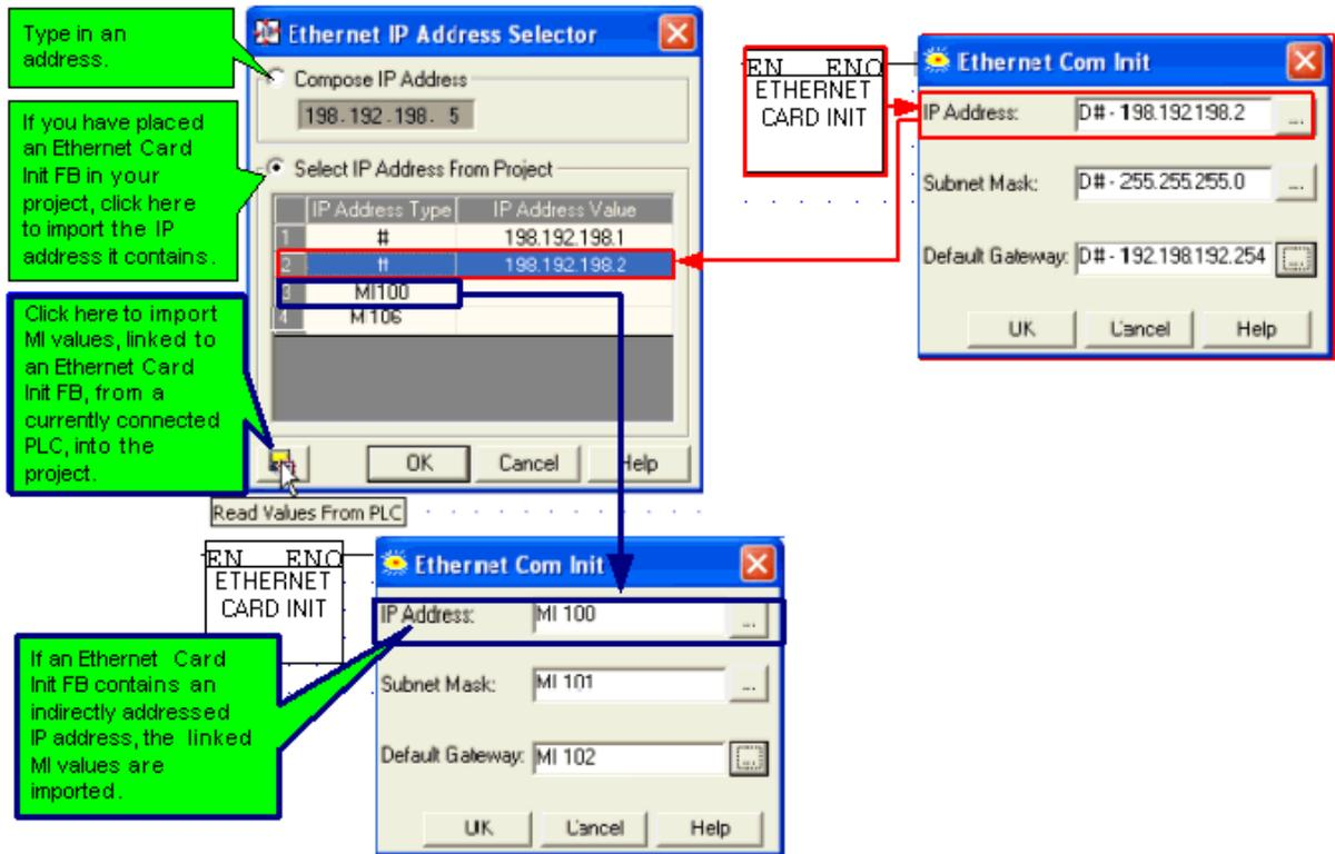
**Note •** If you import a Vision's IP, its protocol type (UDP or TCP) and port number are also imported. If you have typed the IP address, you must also type the port number.
