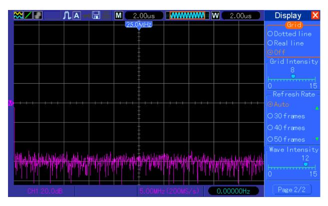
12. In FFT mode "Full span" is higher than Nyquist (sample rate /2 )
