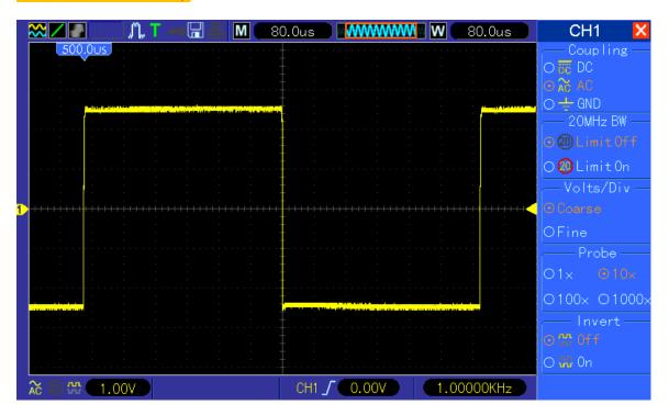
When you now change time base to 40uS/DIV the falling edge (which should be still in the middle of the screen) has been moved to 454uS position (but it should stay on 500uS). The same happens of course with 20uS/DIV.
