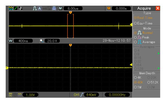
When the Acquisition qould be stopped and restarted or Timebase changed one position forth and back (while Main window is focused) the Main TB and displayed data will be fixed to proper length; no artifacts shown anymore:
