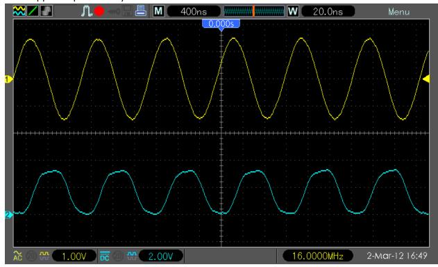
15. Display / Time base scaling strange behavior. When you apply e.g. 1kHz signal, set time base to 80us/DIV and move the waveform to 500us/DIV (bug only in 4/40k memory depth, 512k/1M/2M works fine):
