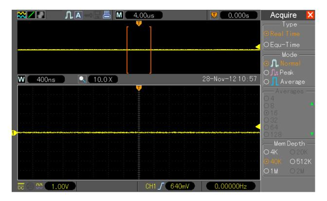
With 2 channels enabled this bug **DOES NOT EXIST**, this is because the doubled Main TB value is exactly what it should be for dual channel view:
