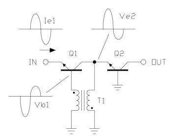
Fig. 3 - Cascade Linearization of the Common-Base Amplfier
