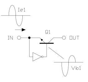
Fig. 2 - Basic Augmentation of the Common-Base Amplifier detects the emitter signal voltage  $v_e$ , amplifies and inverts it, applying the result to the base of  $Q_1$ , resulting in a reduced emitter input resistance  $r_e$ ':
