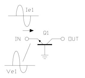
Fig. 1 - Common-Base Amplifier Input Charcteristics
