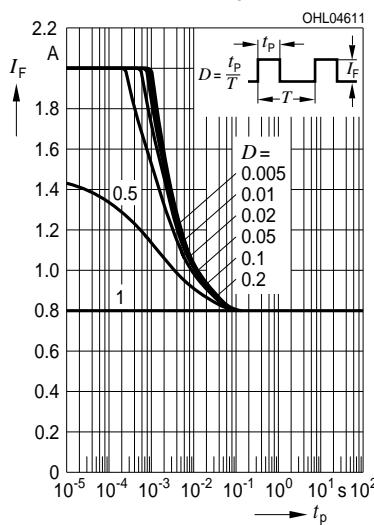
**Zulässige Impulsbelastbarkeit I<sub>F</sub> = f(t<sub>p</sub>)****Permissible Pulse Handling Capability**Duty cycle D = parameter, T<sub>S</sub> = 85 °C
