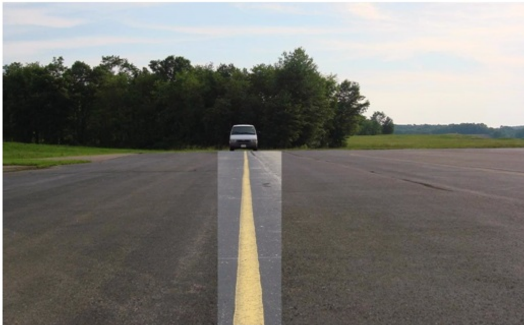
Figure 22: Target object (Van) on the taxiway field placed parallel to the radar
