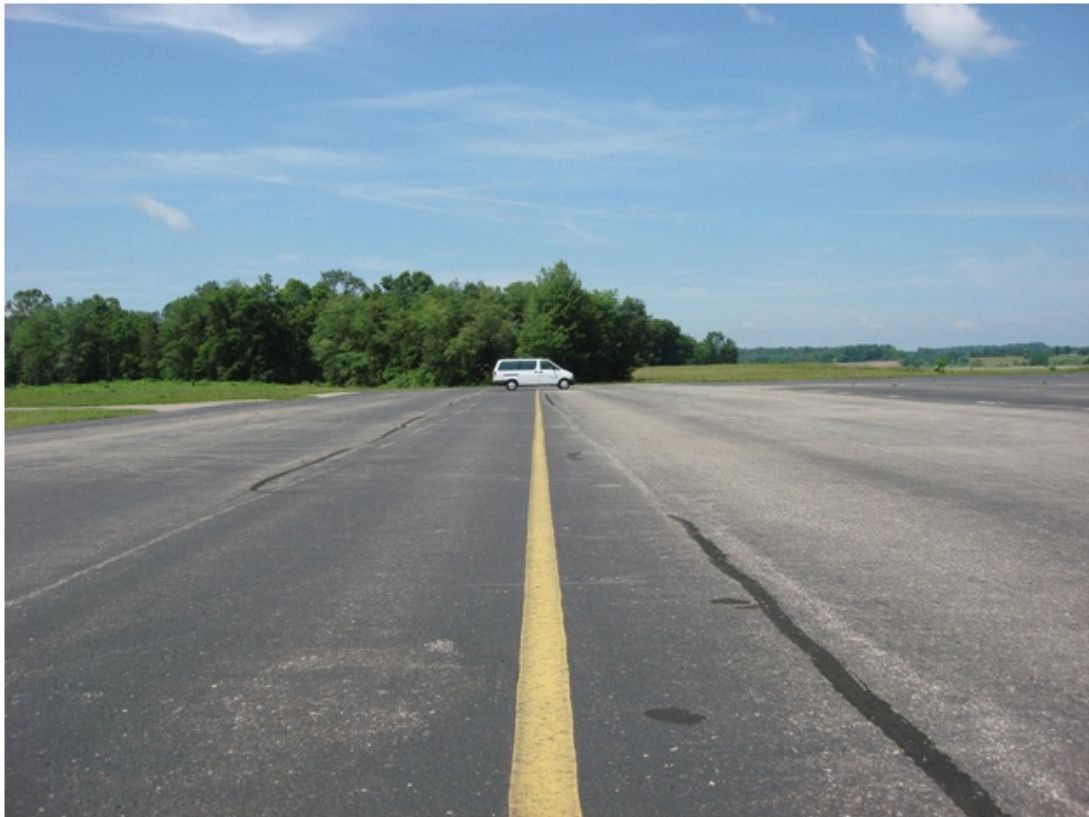
Figure 20: Target object (Van) on the taxiway field placed perpendicular to the radar
