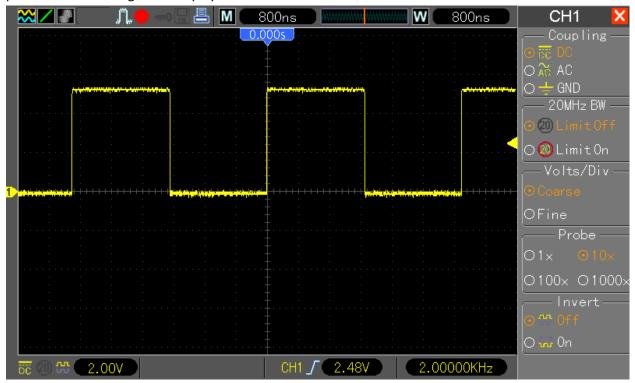
Set DSO to 1ch, 4k memory depth, signal generator to 2kHz square, timebase to 80ns/DIV, dual window mode enabled:
