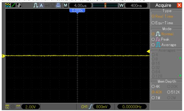
Now when switching to dual window the Main TB is changing to wrong value (here from 4us/DIV to 8us/DIV – actually it will be always doubled in length) and artifacts from "end of buffer" right and left in top window are shown:
