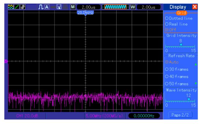
12. In FFT mode "Full span" is higher than Nyquist (sample rate /2 )
