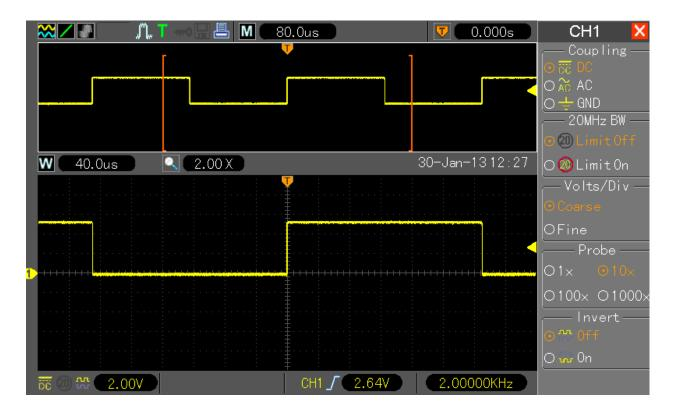
now push "RUN/STOP" button to stop acquisition, the waveform is still ok, can be moved or zoomed, etc:
