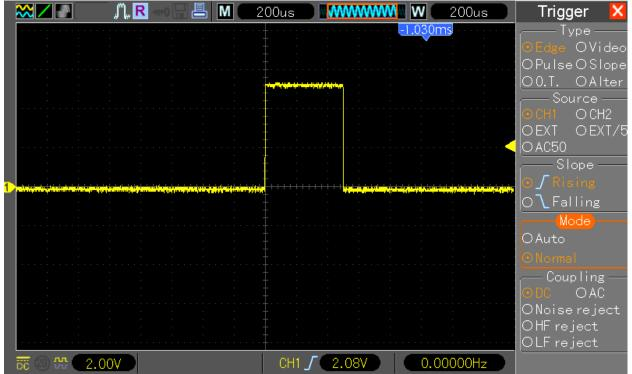
However, when working with acquisition in "Single shot" mode the waveform can be moved together with the trigger indicator:
