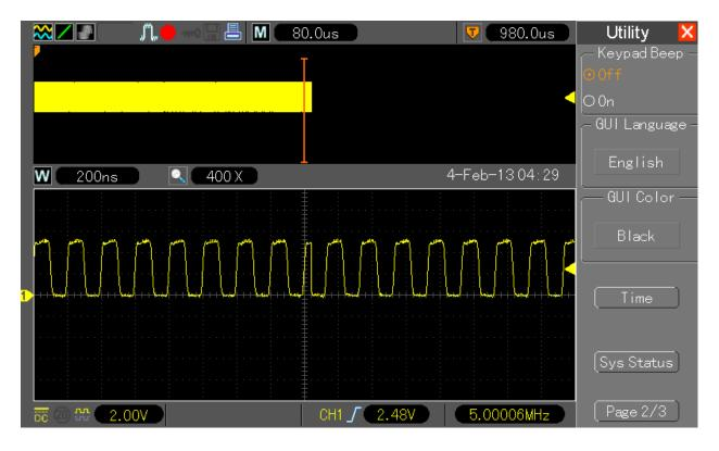
It seems that no matter if the DSO is sampling with 200MS/s, 400MS/s or even 500MS/s (I played a bit deeper) the error is there in 40k, 512k and 1M always somewhere at the end of buffer (up to last  $\sim$  3%).
