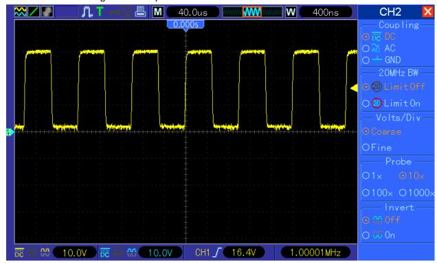
But after changing Timebase (or wave position) one position forth and back the second channel waveform will get displayed and LED gets on :
