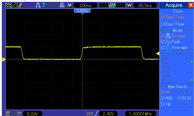
Switch now to 40k, trigger is moved, zeroing of trigger position, selfcalibartion and even factory calibration is not helping. Tested with 83E9 and 83EB FPGA designs:
