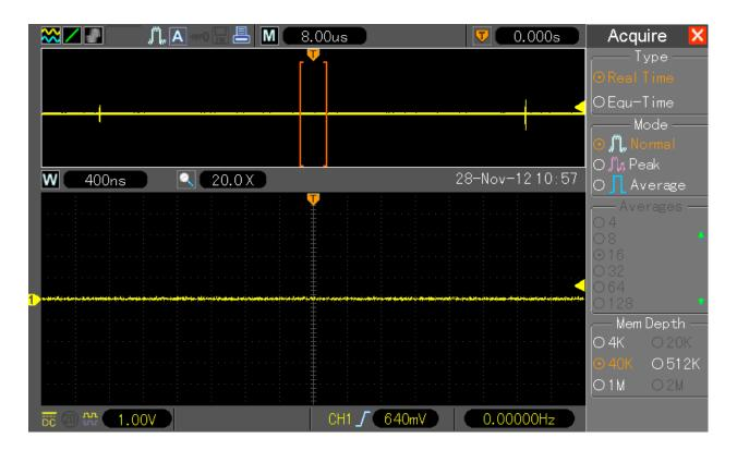
When the Acquisition would be stopped and restarted or Timebase changed one position forth and back (while Main window is focused) the Main TB and displayed data will be fixed to proper length; no artifacts shown anymore:
