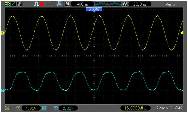
15. Display / Time base scaling strange behavior. When you apply e.g. 1kHz signal, set time base to 80us/DIV and move the waveform to 500us/DIV:
