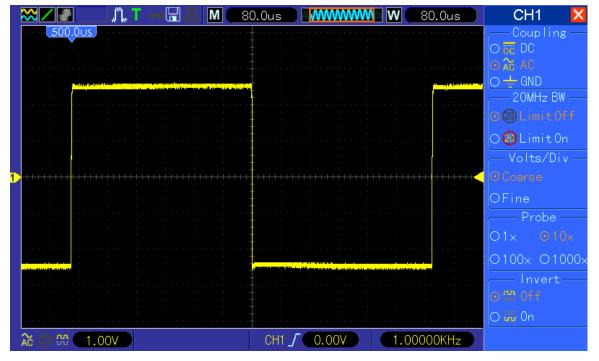
When you now change time base to 40uS/DIV the falling edge (which should be still in the middle of the screen) has been moved to 454uS position (but it should stay on 500uS). The same happens of course with 20uS/DIV.
