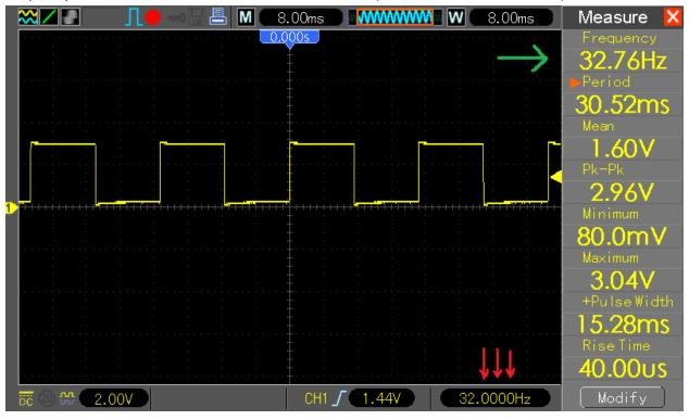
37. With Long Memory enabled (40k, 512k, 1M, 2M?) when the WTB is 400ns/DIV (and lower, up to 2ns/DIV) when enabling second channel the indicator in status line will be already displayed but the waveform is missing. Additionally the CH2 LED is off:
