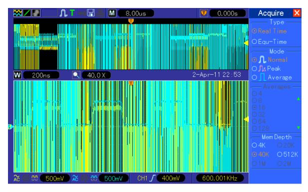
10. In single window mode, sample memory 512k, both channels (ch1, ch2) enabled – when switching to dual window mode artifacts on screen and DSO later crashing and not respondin
