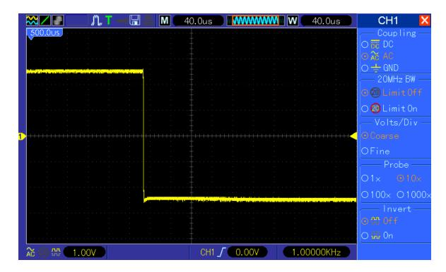
Another example, waveform moved to trigger delayed by 20us:
