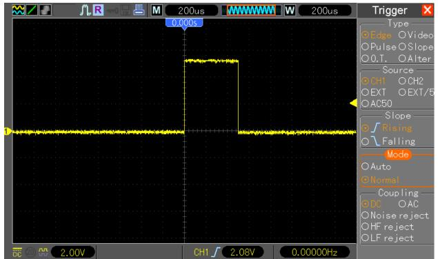
Now when you turn the Horizontal position knob to left or right to change the position, the blue trigger indicator is changing as expected, but the already captured waveform is not moving (which is a bug, it make sense to be able to move already captured waveform while waiting for next trigger event.)
