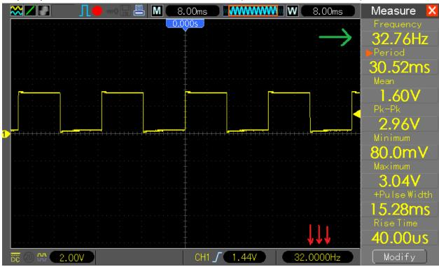
frequency of 32.768Hz – the counter will show 32.000Hz (and Wave measure 32.76Hz).
