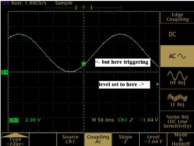
14. For sure a stupid bug, but since you can see when the signal is "wobbling" you can quick change (when necessary) to single channel to observe the waveform with better resolution and without
