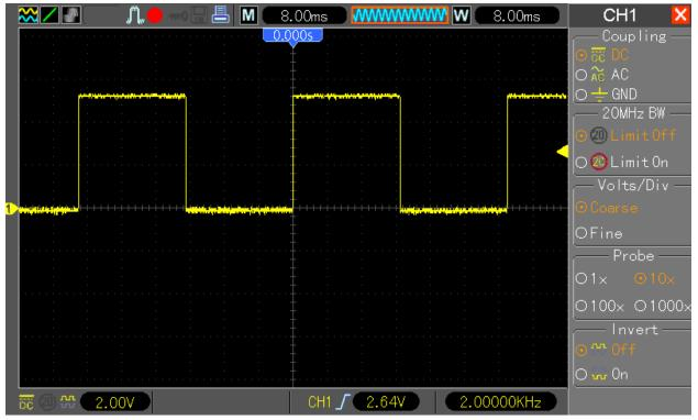
42. Measurement "Delay1-2Rise" and "Delay1-2Fall" displaying too long (wrong) result when the delay is equal zero (no delay):
