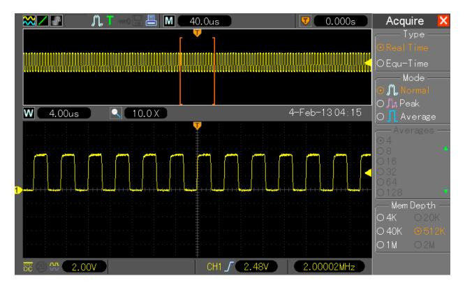
Switch now focus to top window and turn timebase one position up, the display will be refreshed to **proper values**:
