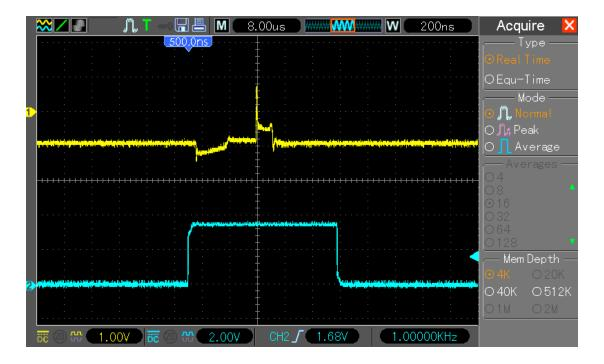
with 4k memory when changing position waveform is moving
