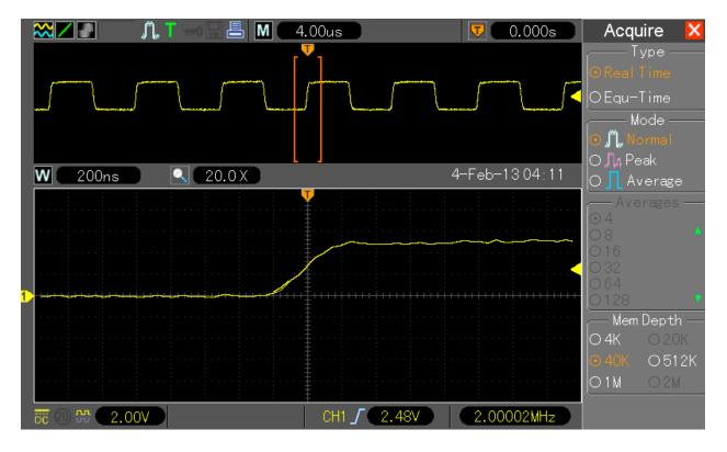
Switch now focus to top window and turn timebase one position up, the display will be now refreshed to **proper values**:
