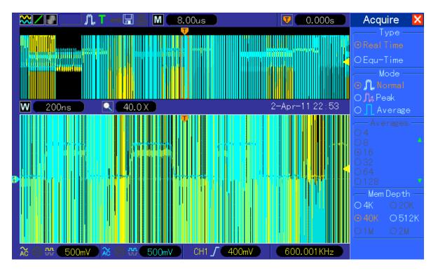
10. In single window mode, sample memory 512k, both channels (ch1, ch2) enabled – when switching to dual window mode artifacts on screen and DSO later crashing and not respondin
