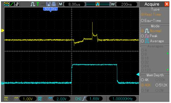
In single window mode, sample memory 40k, both channels (ch1, ch2) enabled – while switching to dual window mode artifacts on screen and DSO later crashing and not responding.
