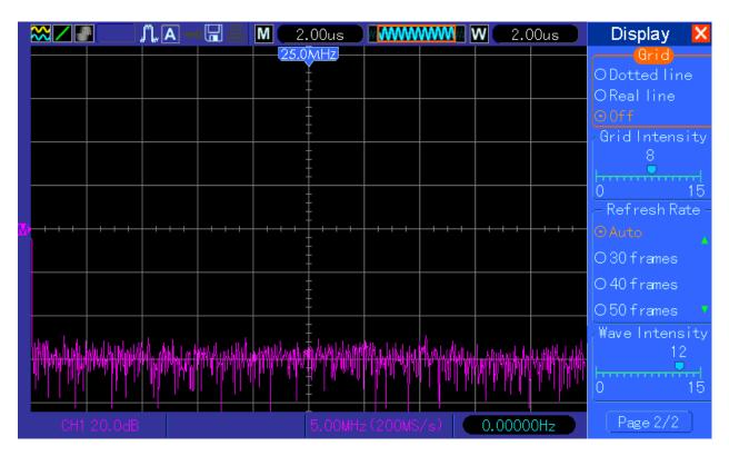
12. In FFT mode "Full span" is higher than Nyquist (sample rate /2)Example: 800ns/DIV, sample rate is 200MSs, full span 125MHz. Easy to fix by enabling from
