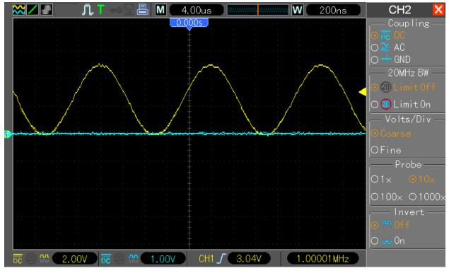
you have to turn again timebase know one up and down position to get display updated to proper value which is in this example 8us/DIV:
