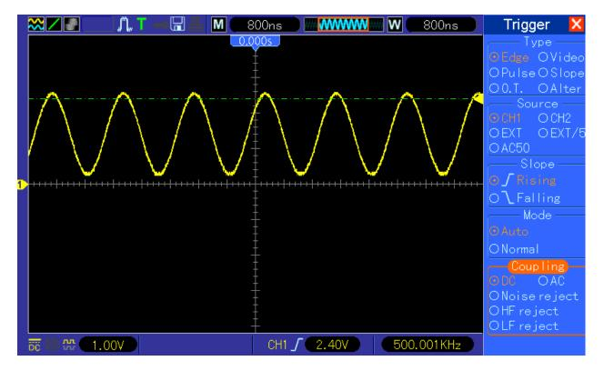
14. Dithering/interpolation filter of waveform too sharp. When enabling both channels (this also occurs in single channel mode and 1GSs, but test signal need to be higher to get same error) and applying for example 16MHz square wave the waveform is switching between proper square:
