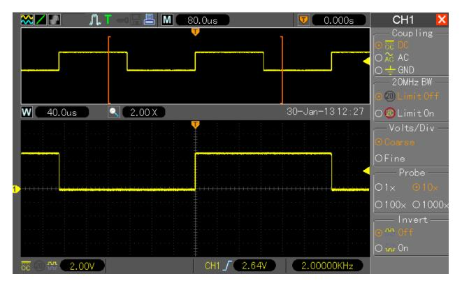
Set DSO to 1ch, 4k memory depth, signal generator to 2kHz square, timebase to 80ns/DIV, dual window mode enabled:
