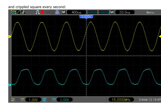
15. Display / Time base scaling strange behavior. When you apply e.g. 1kHz signal, set time base to 80us/DIV and move the waveform to 500us/DIV:
