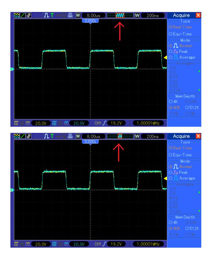
39. Within FFT the information in status bar is not always showing the proper sampling rate, sometimes even jumping from proper to bad value. As the FFT cursor is taking in count the sampling rate, the measure value might be not correct. Example random values in 800ns/DIV
